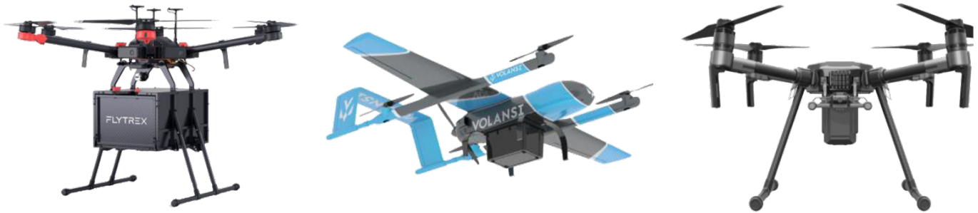
Figure 18. Test vehicles for Causey testing campaign. From left to right, Flytrex FTX-M600P, Volansi VOLY C10 and DJI® m210.
