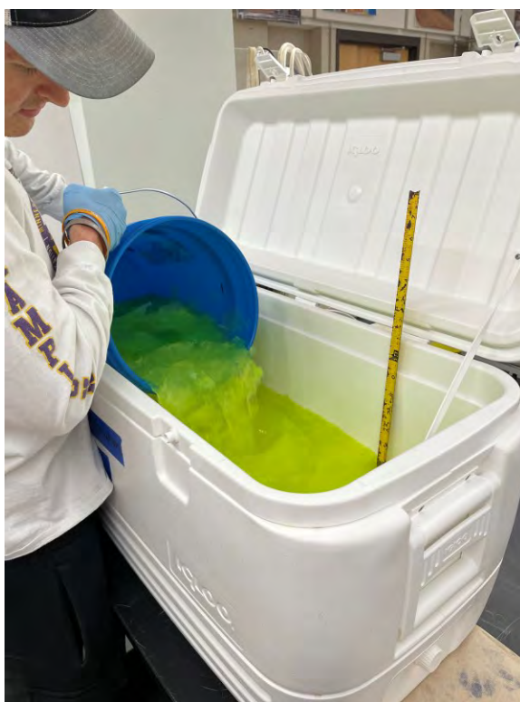
Figure 14. Ice slush composed of glycol – water mixture being placed in a freeze chamber (cooler) at -26 °F.
