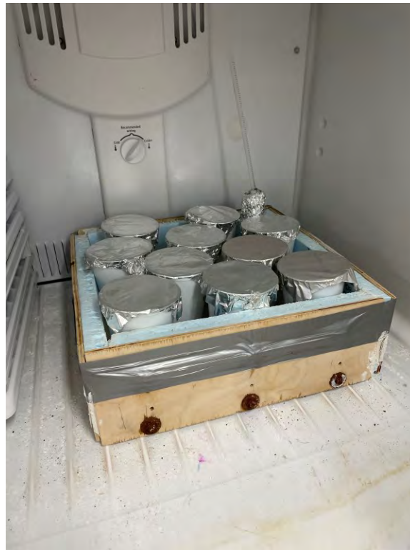
Figure 13. Thermal stabilization unit in 0 °F freezer with 10 prepared ice specimens and measurement thermometer.
