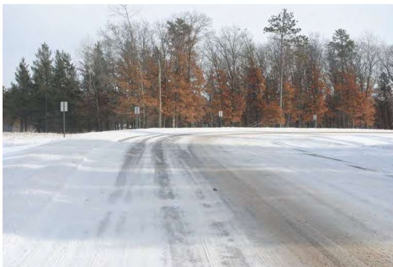
Figure 39. Typical results (EB2 with 200 lbs/LM rock salt and 25 gal/LM 70:30 prewet). From top to bottom: 4 minutes, 34 minutes, and 57 minutes after application.
