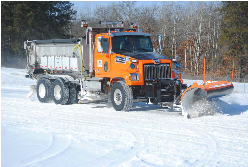
Figure 35. Plowing left on perimeter track; no treatment.
