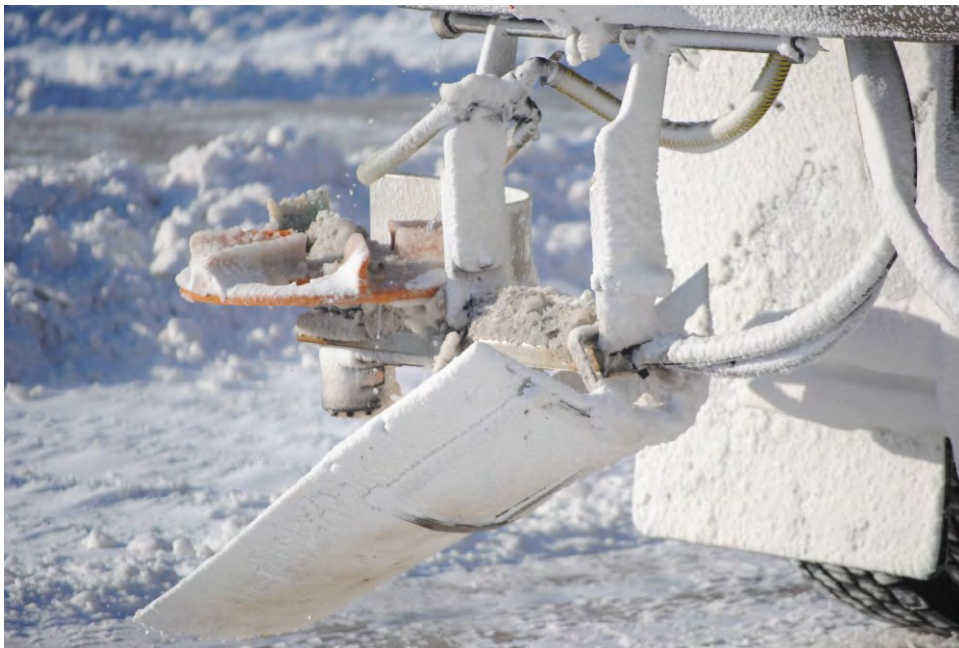
Figure 28. Treatment attempt on SKID 3; note no application of material due to equipment freeze up.
