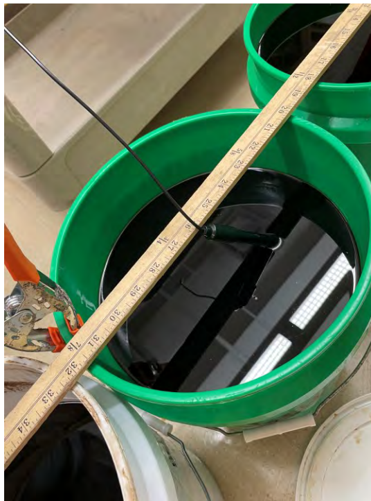
Figure 2. Conductivity testing: measurement probe suspended in sample within bucket.
