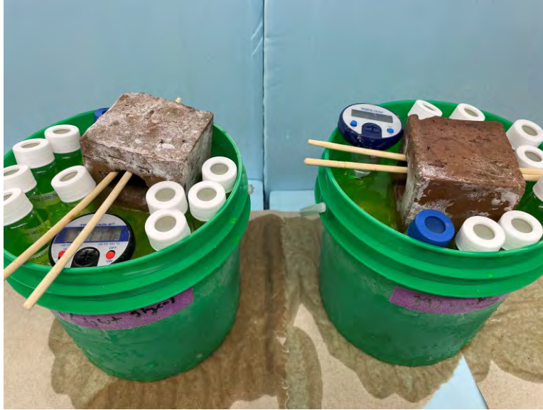
Figure 8. Bucket freeze chambers with supporting brick and specimen vials; temporarily removed from 0 °F to inspect and observe vial specimens.
