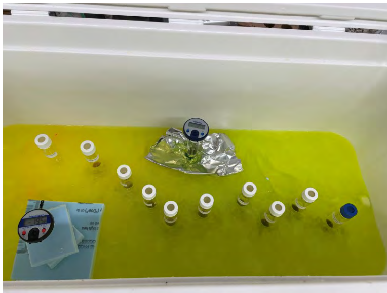
Figure 9. Direct insertion method of chilling specimens to a target temperature; placement in a cooler freeze chamber with floating thermometers.
