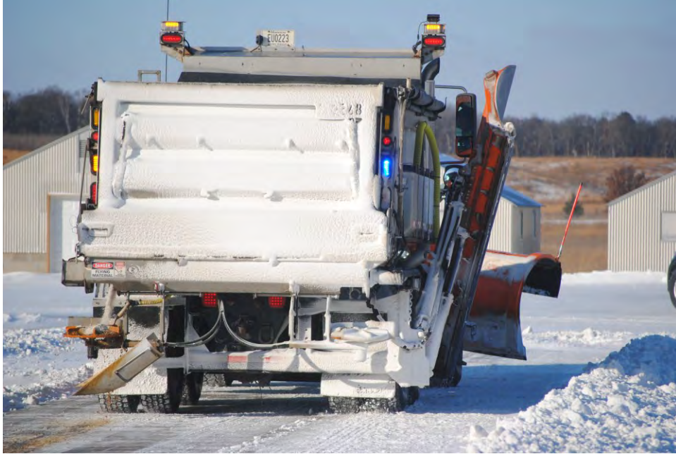
Figure 29. Treatment on SKID 4; note overapplication of material due to equipment freeze up.
