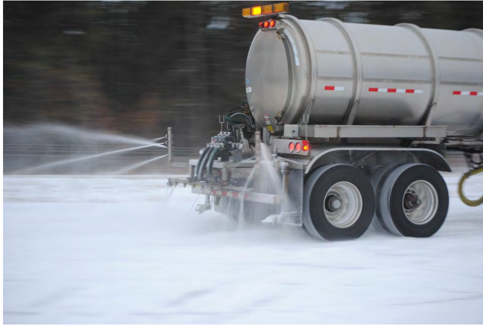
Figure 20. Adding moisture to the snowpack by tanker truck spray application to snow cover of perimeter track.
