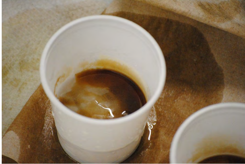
Figure 17. Melted ice brine on top of ice specimen (removed from cold chamber and placed on insulating foam for duration of measurement procedure).
