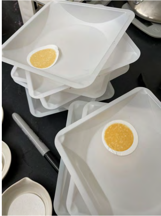
Figure 4. Filters retaining suspended solids.
