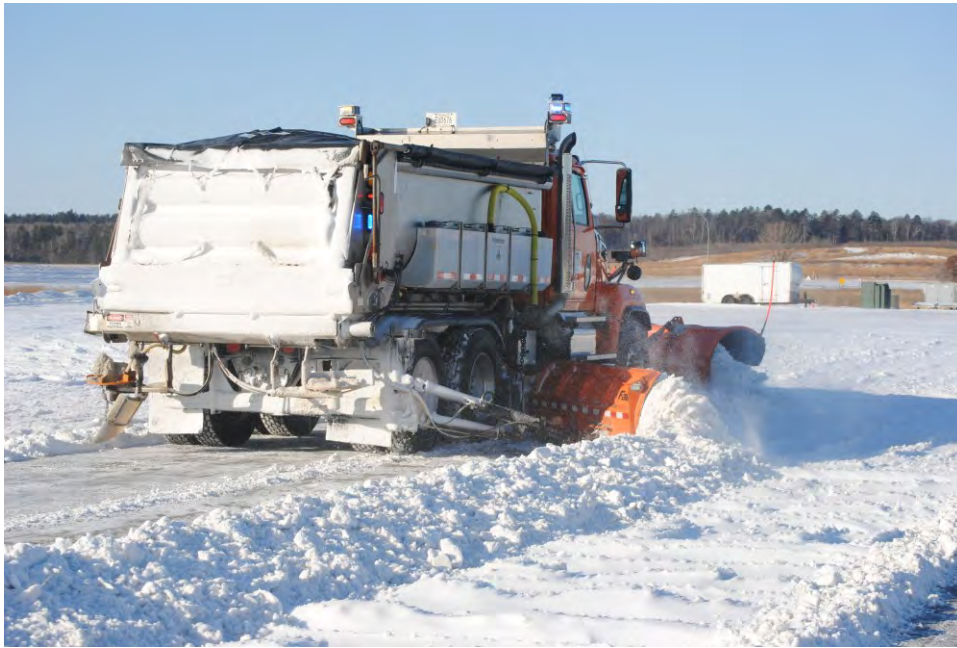
Figure 25. Plowing of skid pad treatment lane; no treatment at first.
