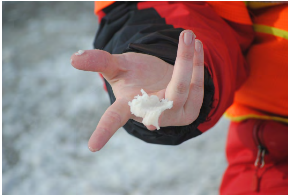
Figure 33. Weak and moist condition of residual snow on skid lane after treatment.
