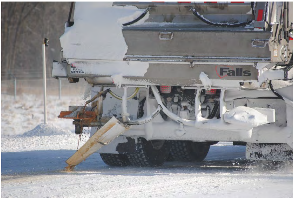
Figure 37. Deicer application on perimeter track by truck plowing to right side.
