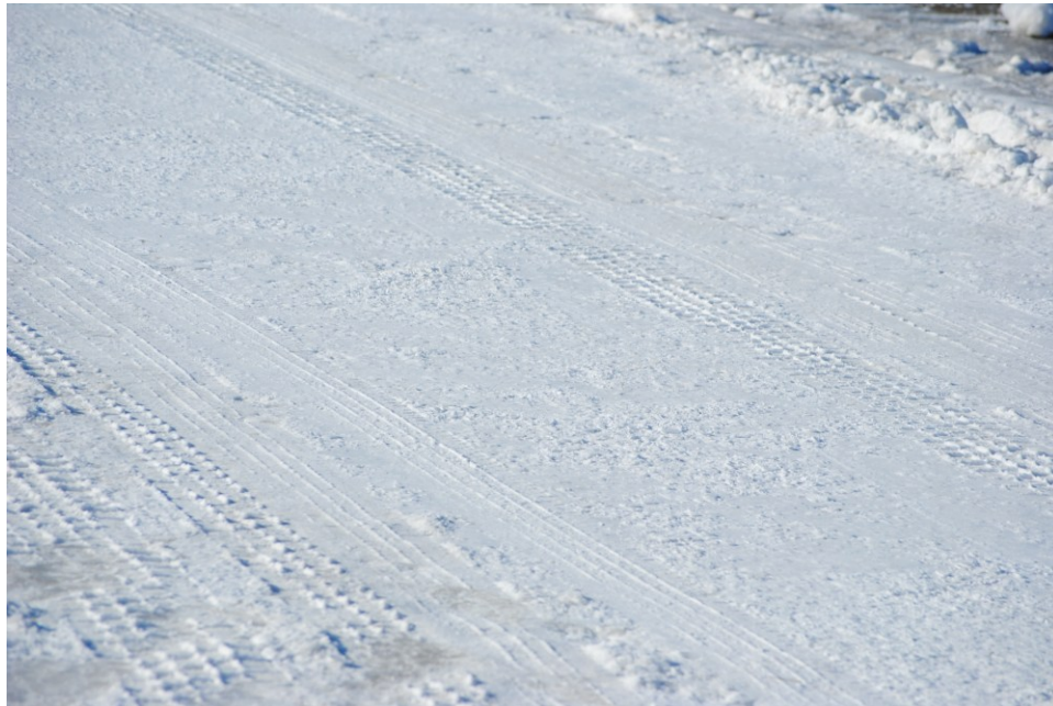
Figure 5. Conditions at the skid pad, location Uniform just after the test beginning.
