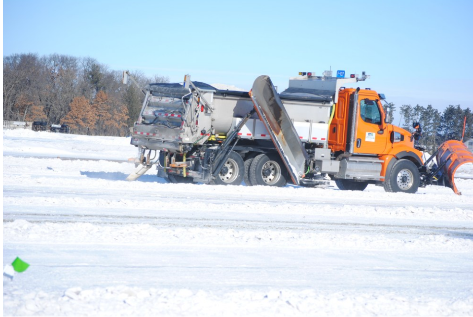
Figure 6. Deicer being applied to a test lane at the skid pad.
