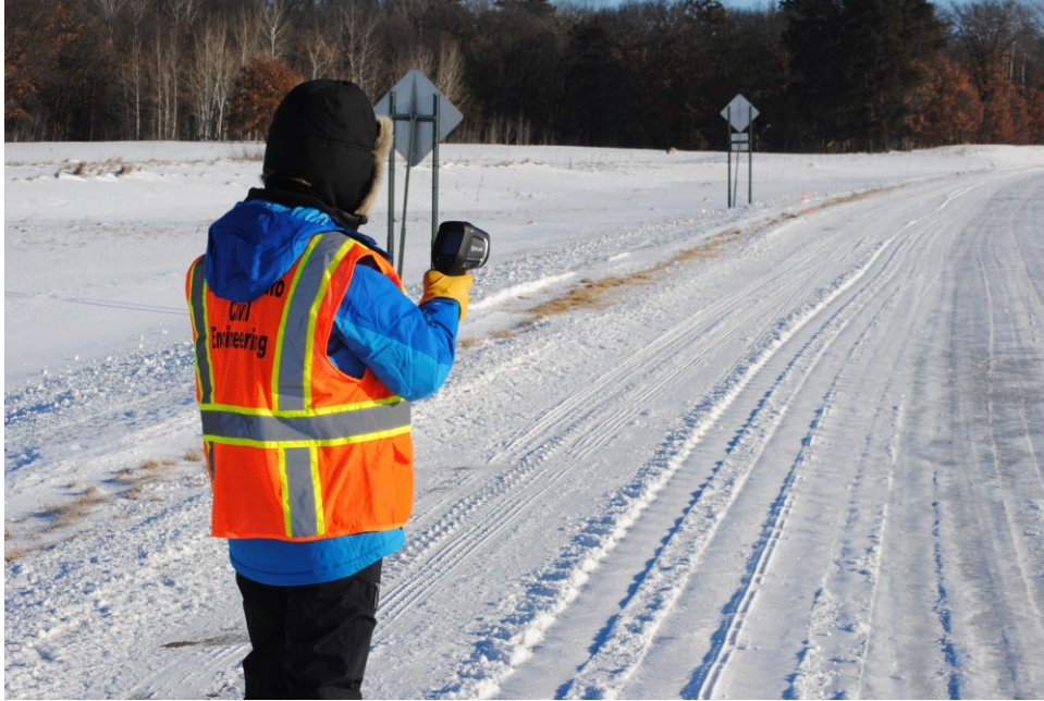
Figure 9. Observations of roadway surface temperature being collected through thermography. Visual observation of snow and ice condition on the roadway surface were collected separately by photography.
