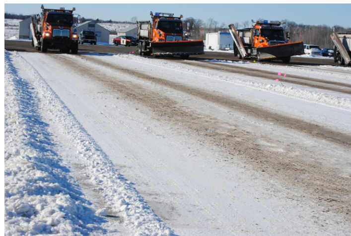
Figure 12. Typical skid pad lane testing results (Quebec with 200 lbs/LM rock salt and 15 gal/LM 70:30 prewet delivered as liquid to the chute). From top to bottom: 5 minutes, 25 minutes, and 47 minutes after initial application.
