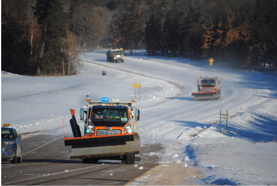
Figure 7. Plow trucks returning from treatment application on perimeter roadway; note MSU research personnel as passenger “ride alongs” to guide treatment location and confirm rates and amounts.
