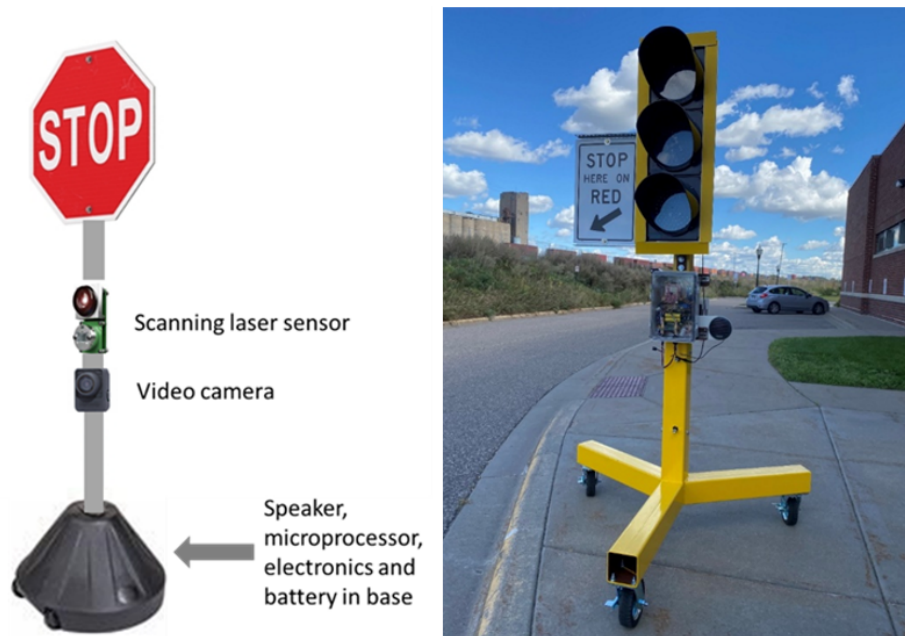
Figure 3.1 (left) Smart sign envisioned at proposal submission; (right) Phase 1 prototype developed from initial user inputs.
