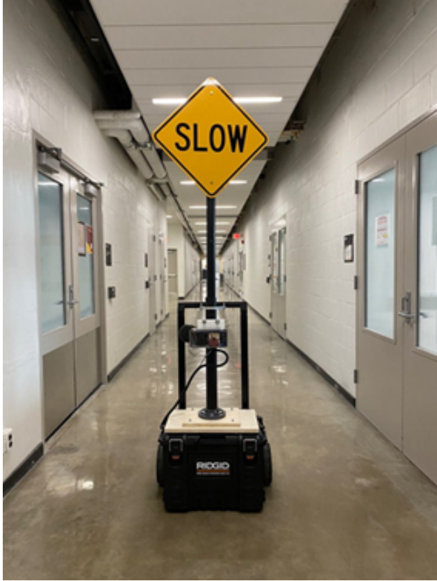
Figure 2.2 Photograph of instrumented sign being used with a taller height, showing adjustability of desired height
