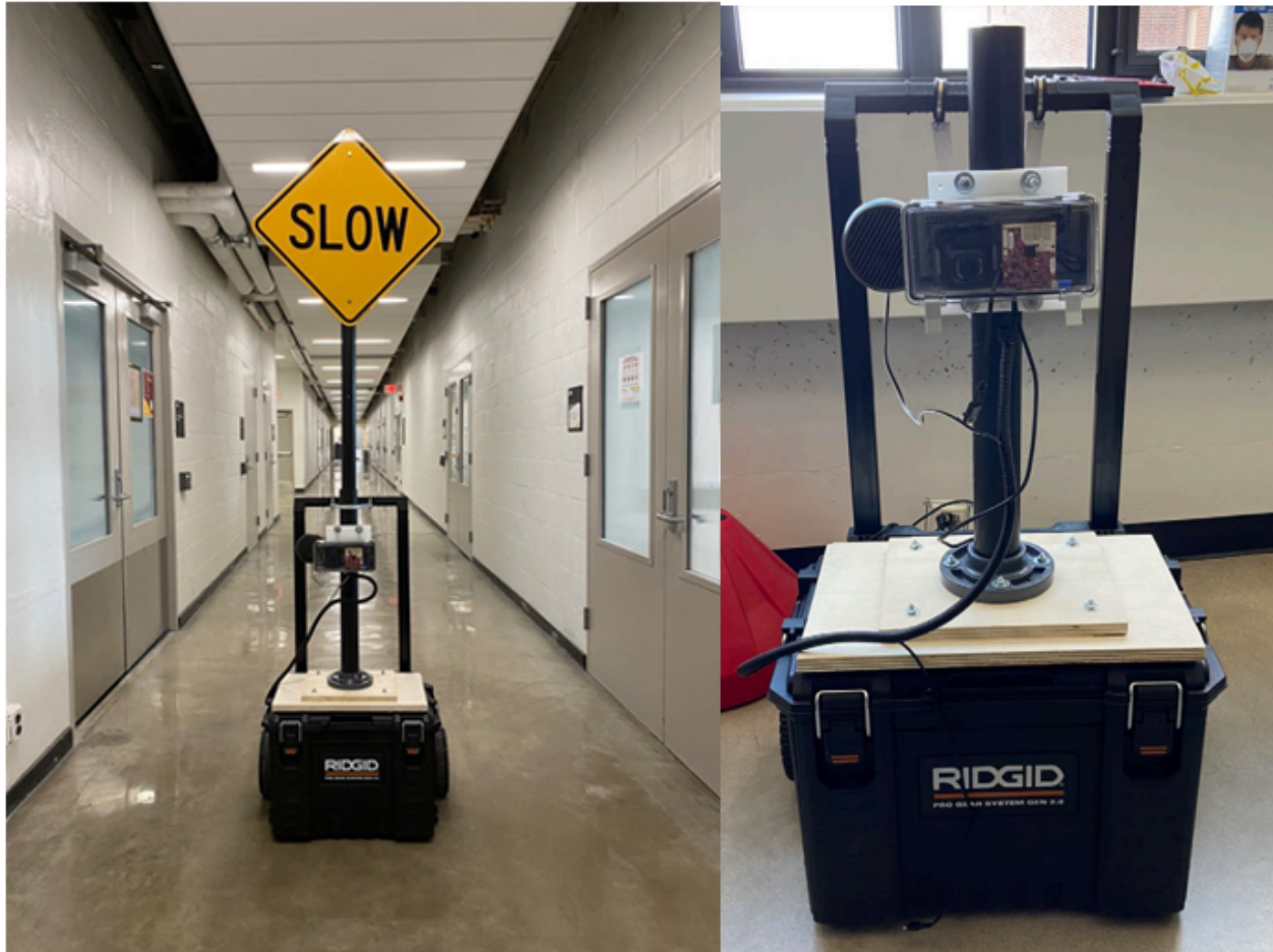
Figure 3.2 (a) Gen 2 prototype developed in Task 2; (b) radar and electronics decoupled from the STOP/SLOW sign.
