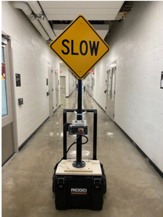
Figure 2.1 Photograph of instrumented sign for use by flag workers
