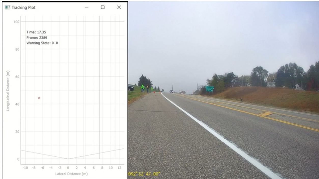
Figure 3.11 Screenshot of radar-tracking animations synchronized with video.
