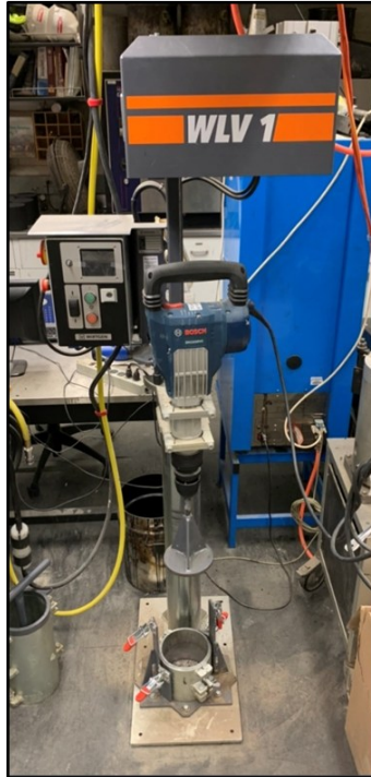
Figure 3-7 Wirtgen Vibratory Hammer (Model WLV1)
