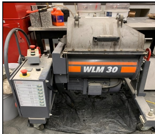
Figure 3-6 Wirtgen Pugmill Mixer (Model WLM30)
