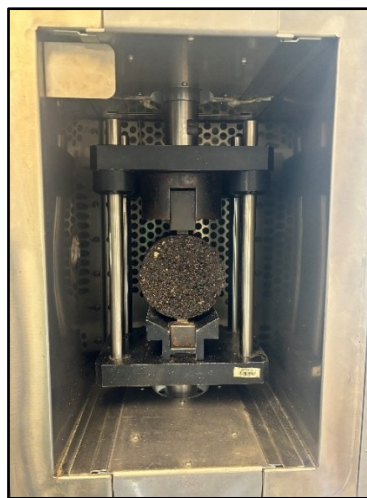
Figure 3-9 Indirect Tensile Strength Test Setup
