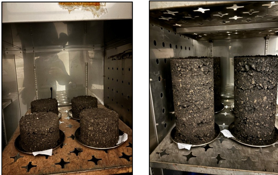
Figure 3-8 Specimen Curing in Oven (at 25°C/77°F)
