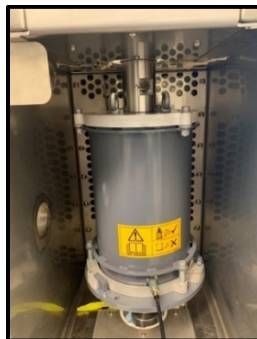
Figure 3-13 Triaxial Test Setup in the Universal Testing Machine
