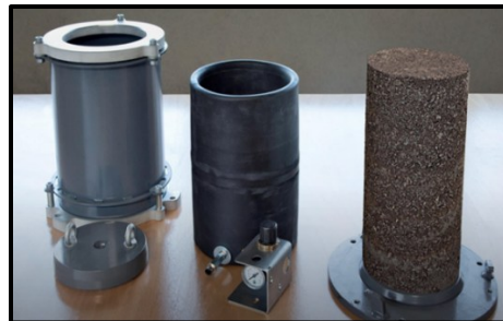
Figure 3-12 Components of Triaxial Testing Device (Mulusa, 2009)
