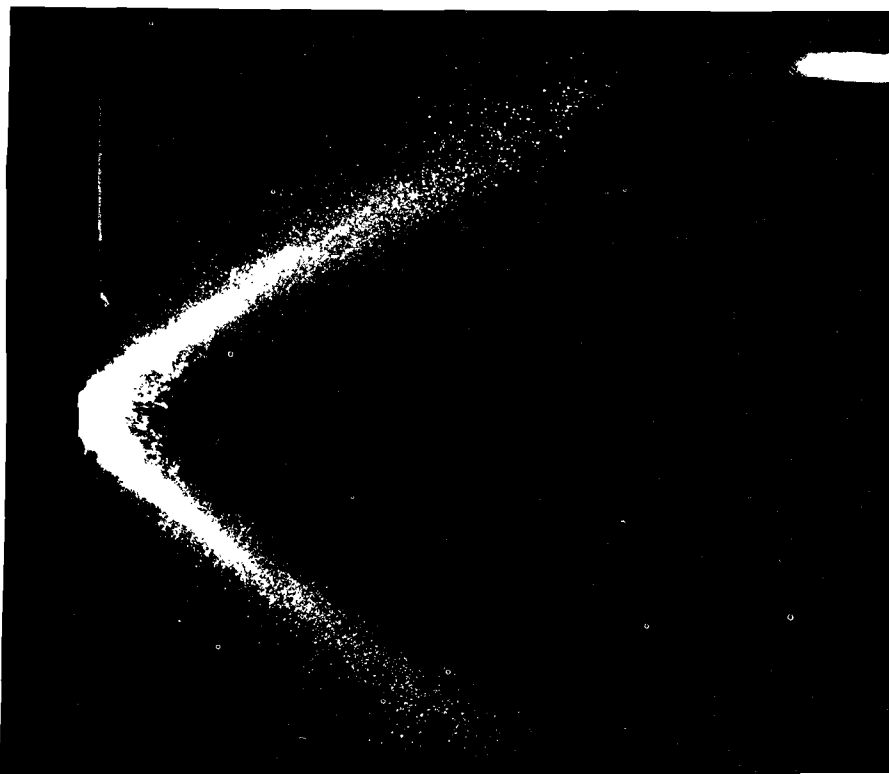
Figure 1-10 ORIGINAL IMAGE OF A JET A FUEL SPRAY AT THE TAKE-OFF CONDITION
