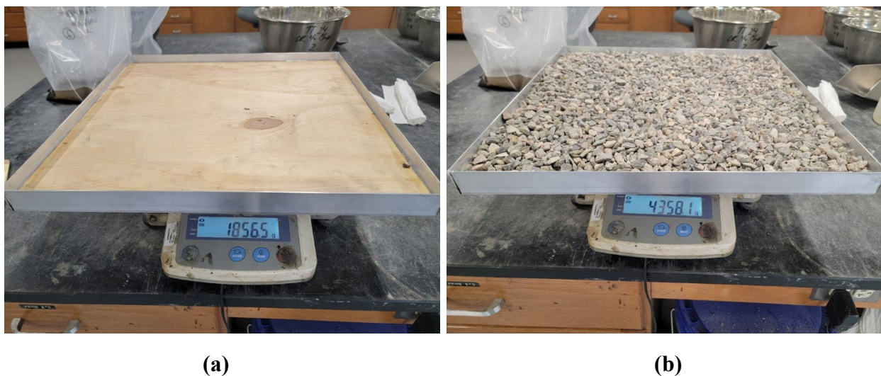
Figure 13. Illustration of Board Test: (a) Empty Board; (b) Board Filled with Aggregate.
