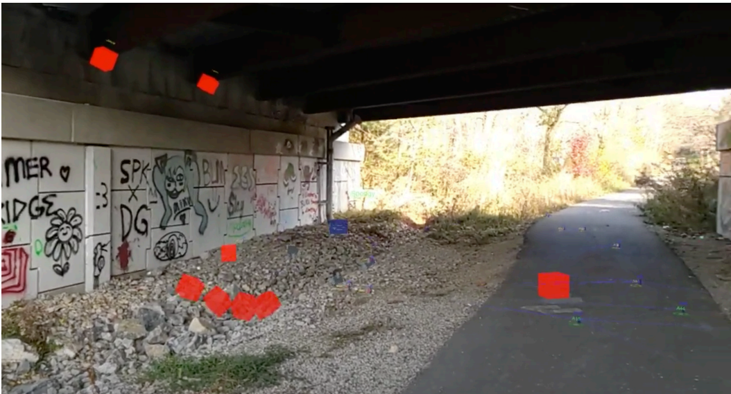
FIGURE 2 We also tested WLT to confirm offline tracking persistence. Virtual objects (red boxes and blue/green markings along paved path) maintained their position between
