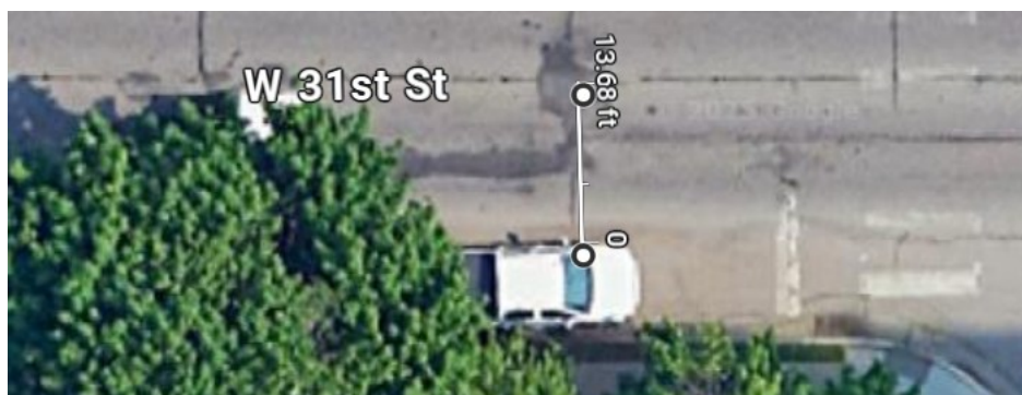
Figure 4.12 Overhead picture of Pillsbury & 31st, with a distance estimation of the lane width from a vehicle parked on the street to the middle of the street. Images and estimation taken from Google Maps ©.
