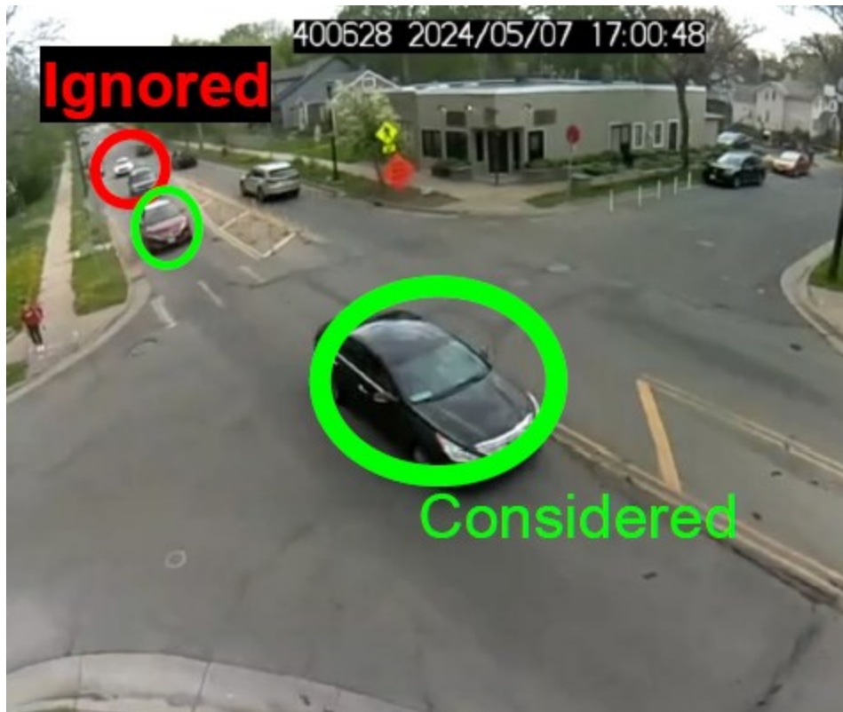
Figure 2.1 Filtering of vehicles following too closely (red circles), while free-flowing traffic (green circles) are considered for speed analysis.
