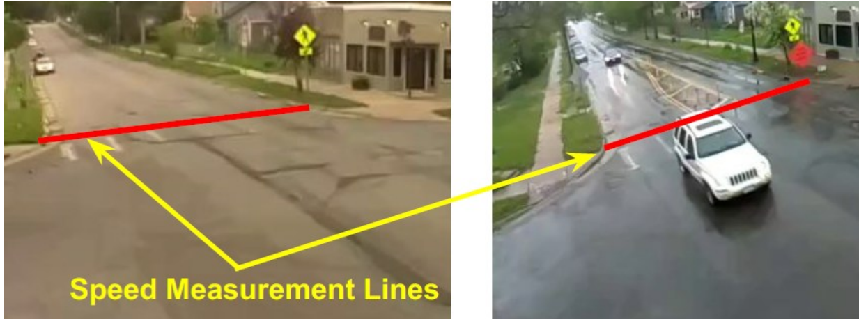
Figure 2.2 Speed averaged over one second is measured at the indicated red lines. The line generally aligns with the pedestrian crossing path.
