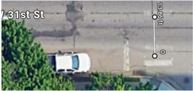
Figure 4.13 Overhead picture of Pillsbury & 31st, with a distance estimation of the lane width from the approximate location of the leading bollard in the temporary curb extension to the middle of the street. Images and estimation taken from Google Maps ©.
