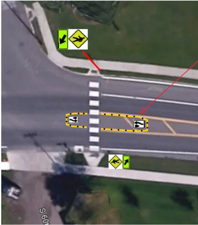
Figure 5.3 An example of a quick-build or temporary pedestrian refuge island installed in MnDOT District 1. Image provided by MnDOT.
