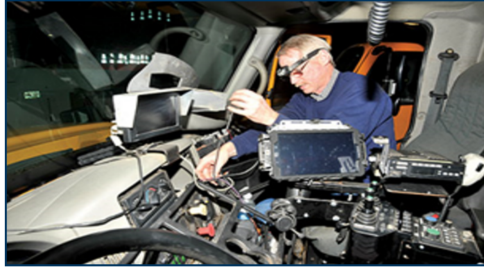
Figure 7: A Member of the WYDOT Installation Crew Installs the Onboard Units
