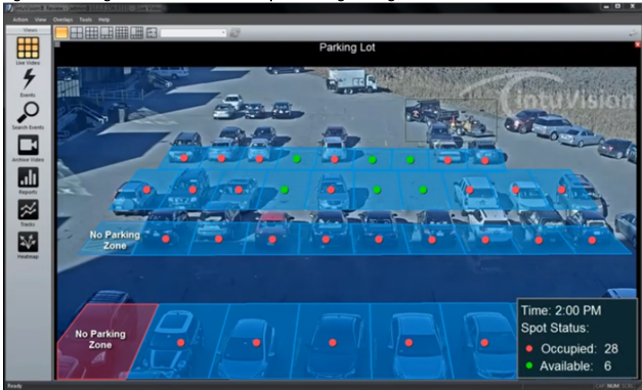
Figure 10. Intelligent Video Software Example Tracking Parking Utilization
