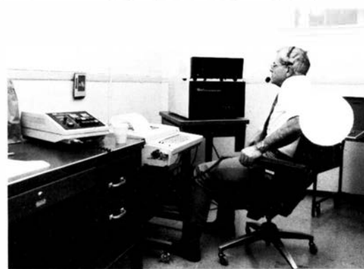
NAFEC's Dr. Donald W. Connolly has been developing a computer-operated Utterance Recognition Device (URD) that FAA hopes can be programmed to recognize human speech, thus permitting pilot briefings and filing of flight plans directly with a computer under the future FSS automated system. This would reduce the need for personal pilot briefings.
