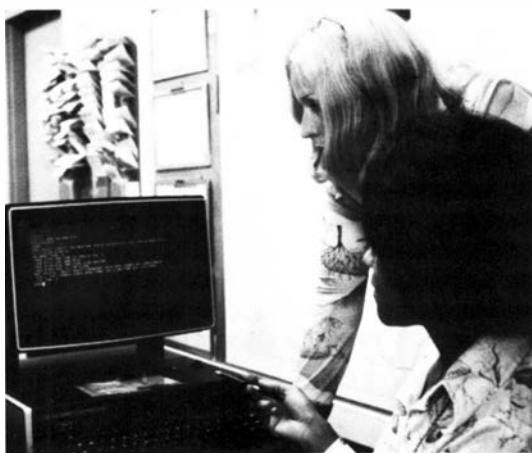
The prototype of an interim modernization now being installed at 150 busy FSSs is at the Chicago FSS. It consists of a CRT display and input device, a small computer updated by the Weather Message Switching Center in Kansas City and a backroom bank of television cameras that transmits weather facsimile maps to the CRTs at specialists' positions.
