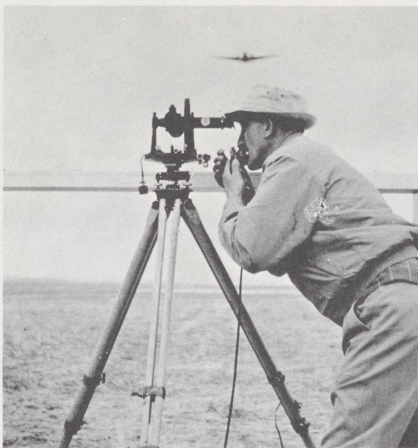
Flight check aircraft making a localizer center-line run for the Colorado Springs, Colorado Instrument Landing System (ILS).
