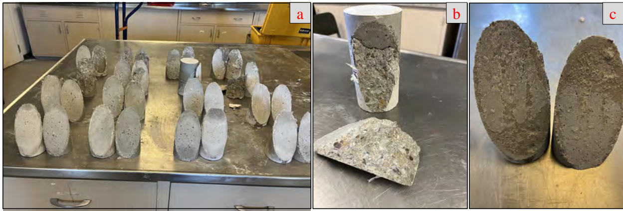
Figure 4.12. a) PVE-PC specimens after testing b) Typical example of bond failure with substrate cracking c) Typical example of pure bond failure
