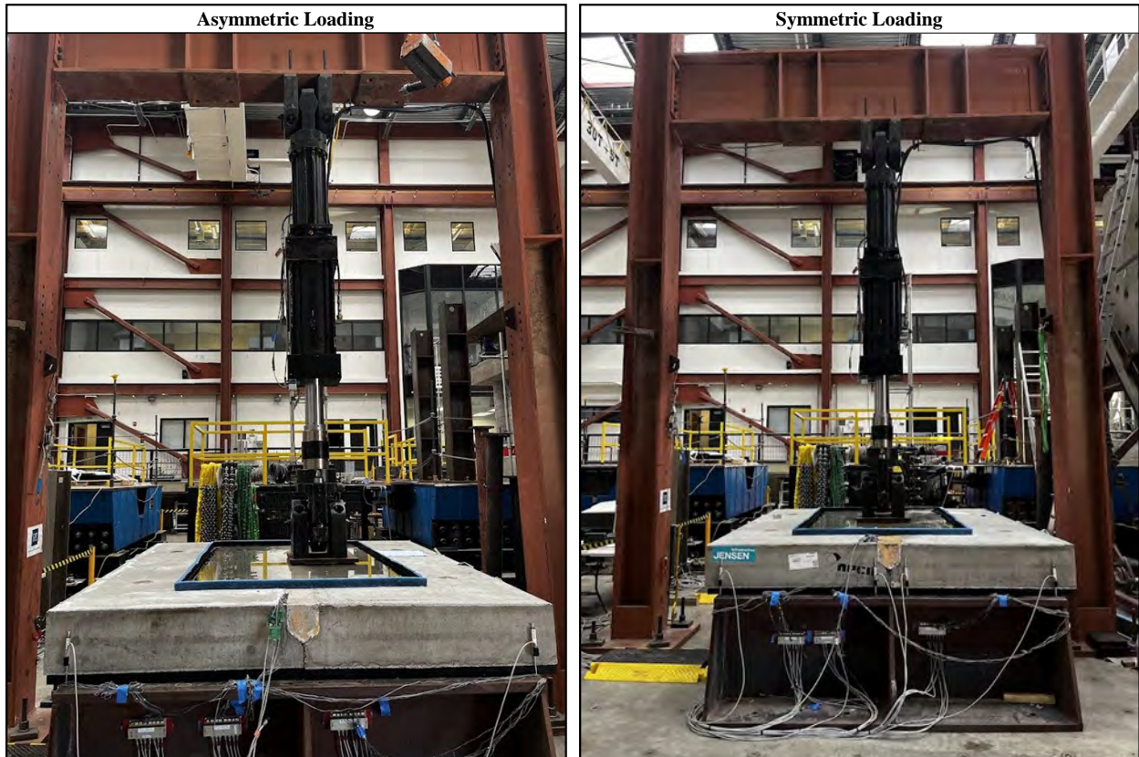
Figure 2.15. Actual test setup with asymmetric loading adjacent to the joint and symmetric loading on top of joint
