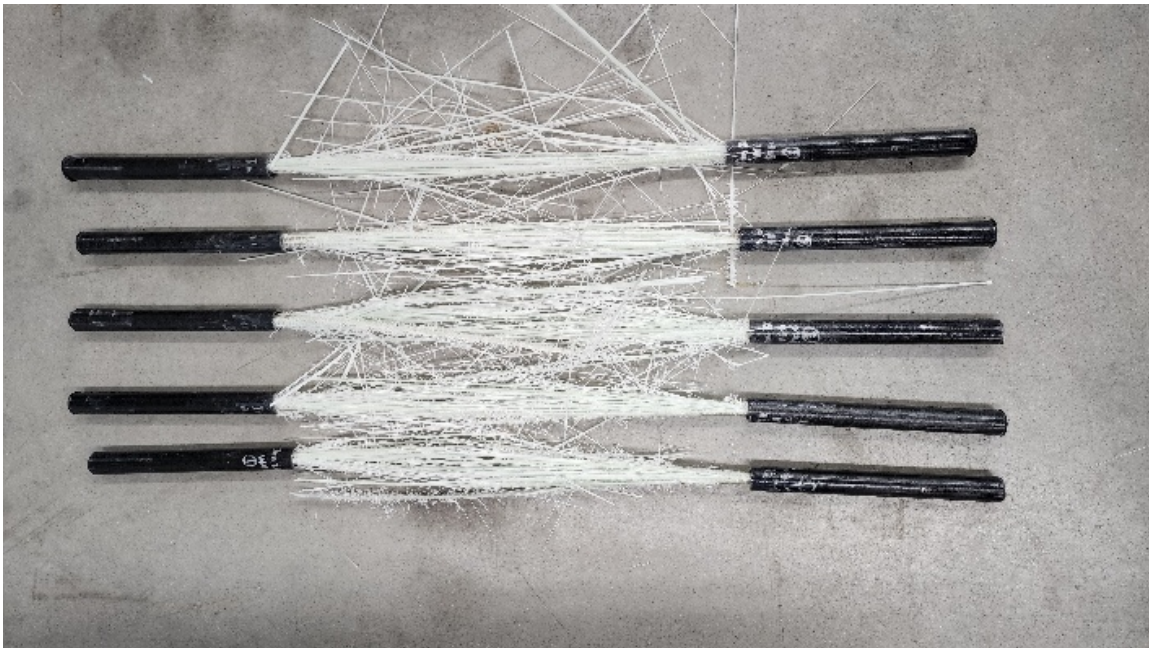
Figure 4: Failed thermoset specimens from tension tests.
