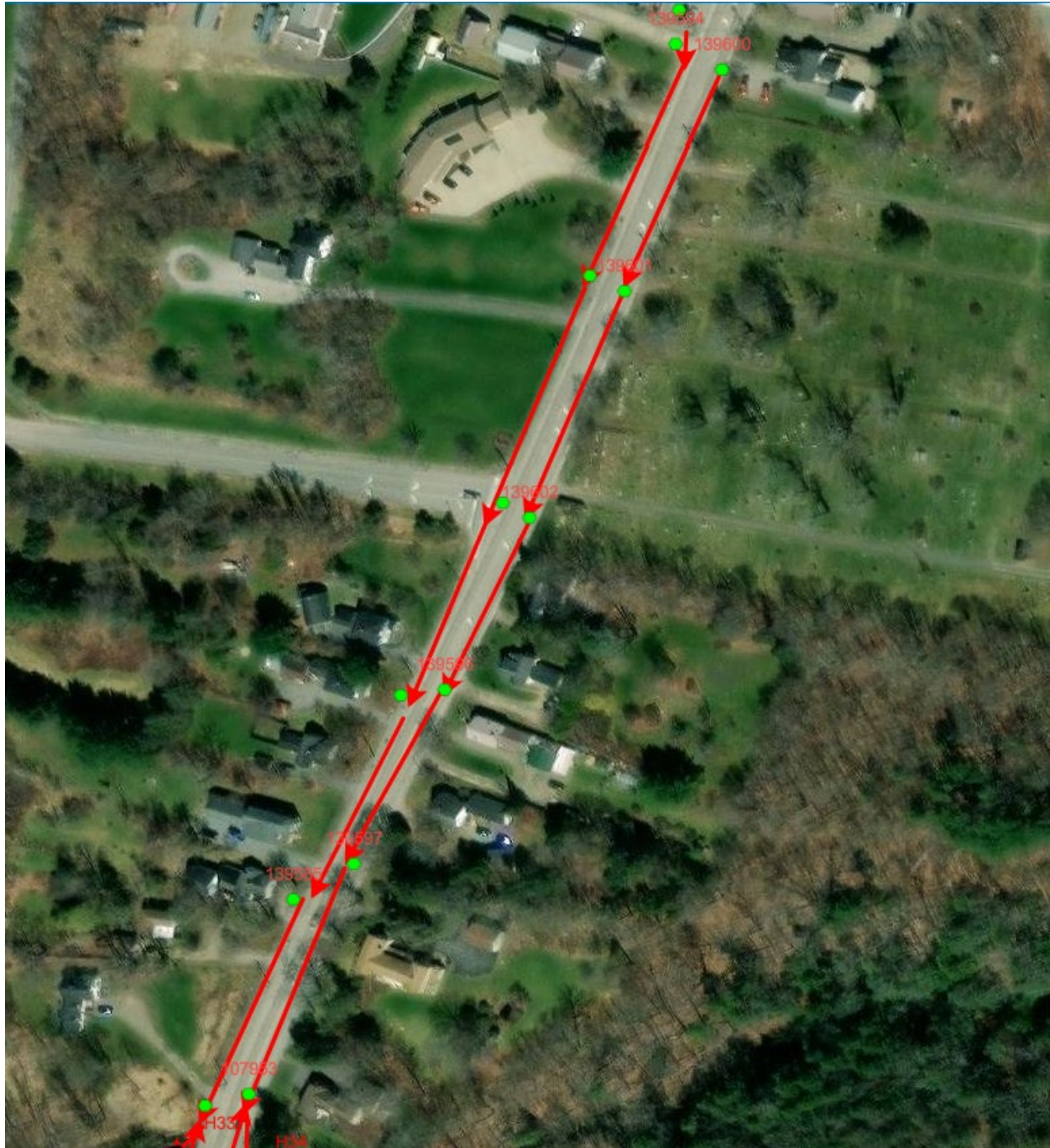
Figure 9: South Hamden closed, inline drainage system (red lines). Monitoring location 2 is at the manhole (green dot) in the lower lefthand of the figure.
