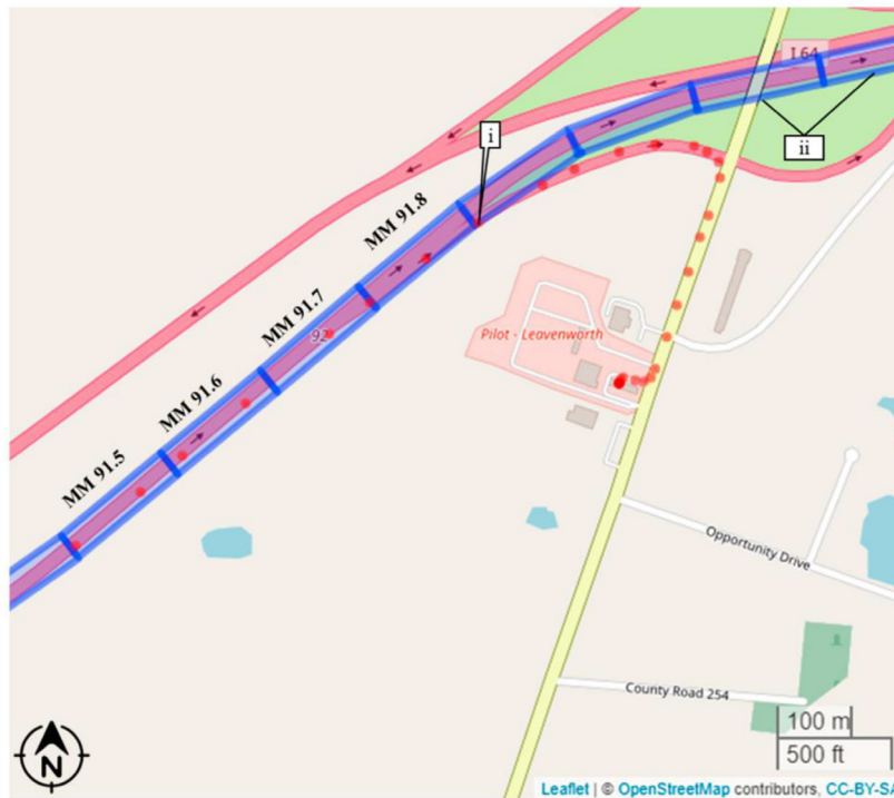
Figure 4.4 Sample CV Trajectory Departing I-64 at Exit 92 Showing Methodology for Detecting Exit Usage (Desai et al., 2022a).
