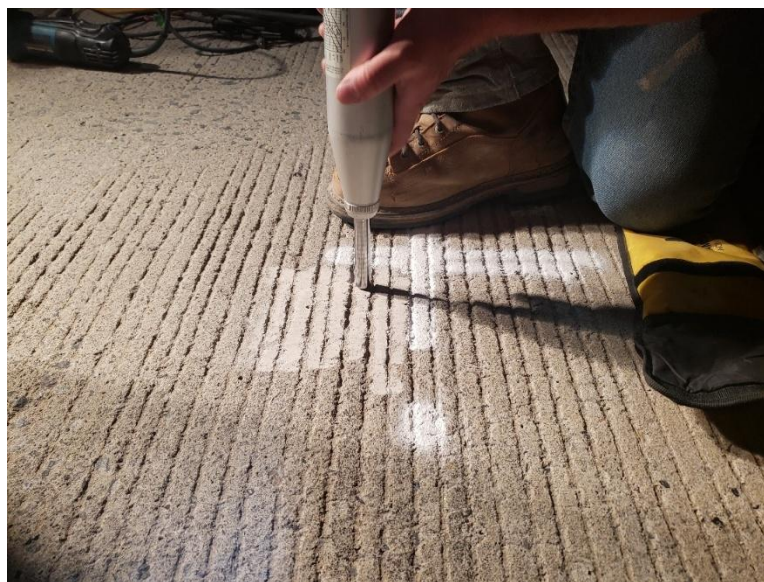
Figure 3.6 Schmidt rebound hammer testing.
