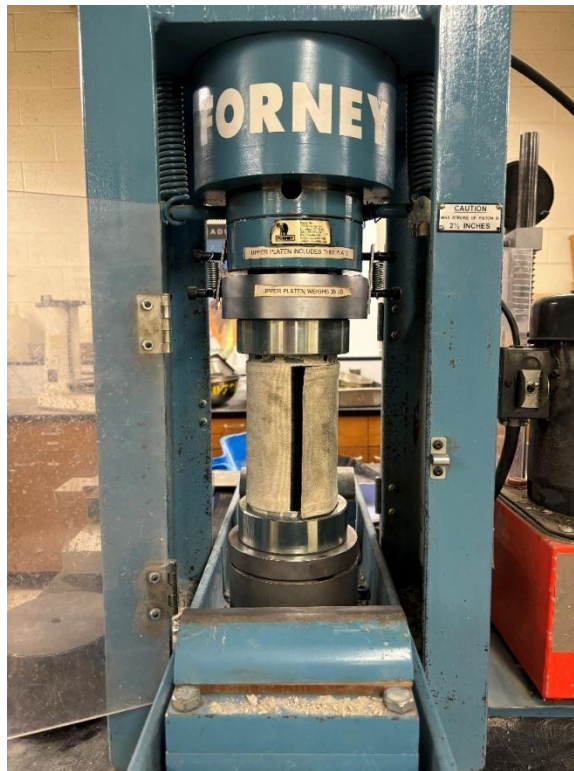
Figure 3.12 Compressive strength testing.
