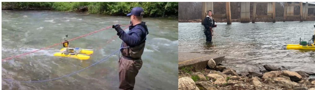
Figure 65: Tethered test in rapidly flowing water.
