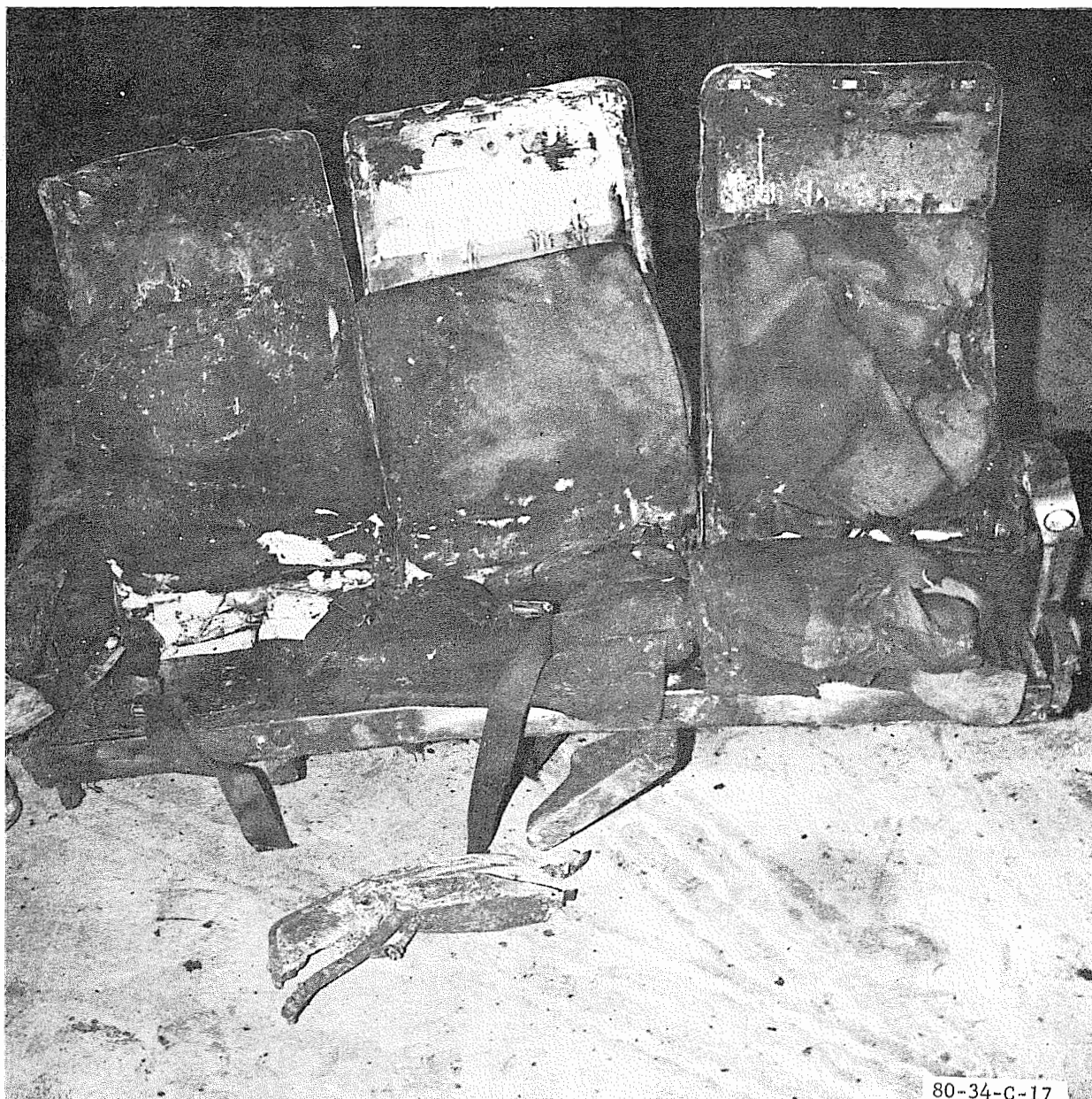
FIGURE C-18. N9031U SEAT DEFORMATION AND FIRE DAMAGE
