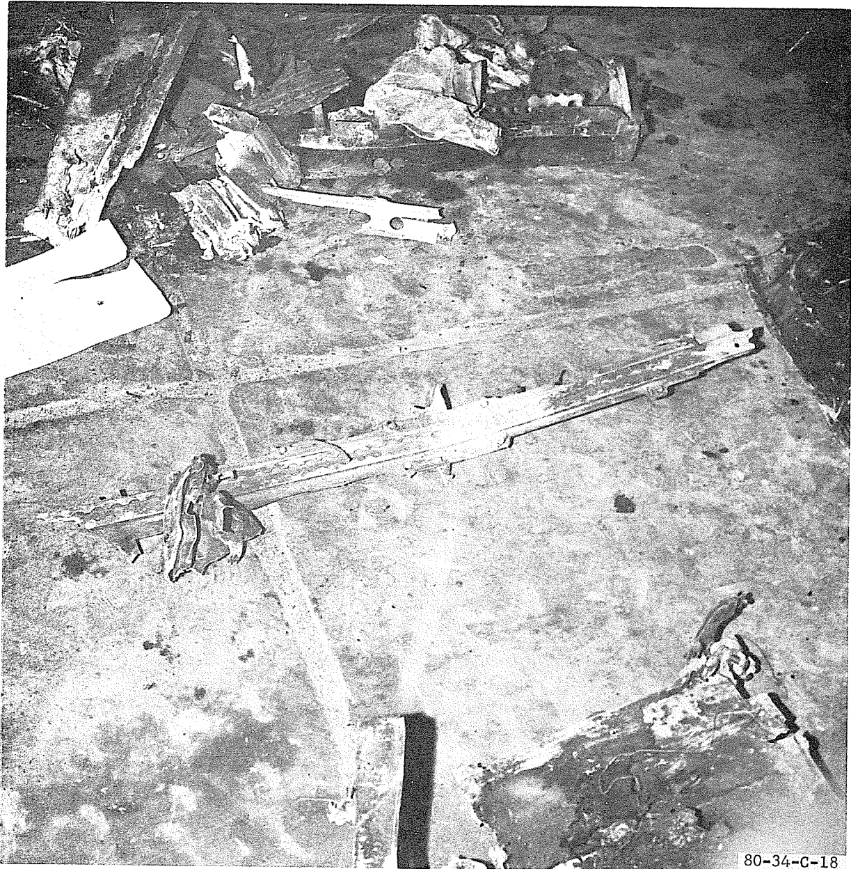
FIGURE C-19. N9031U SEAT TRACK DEFORMATION
