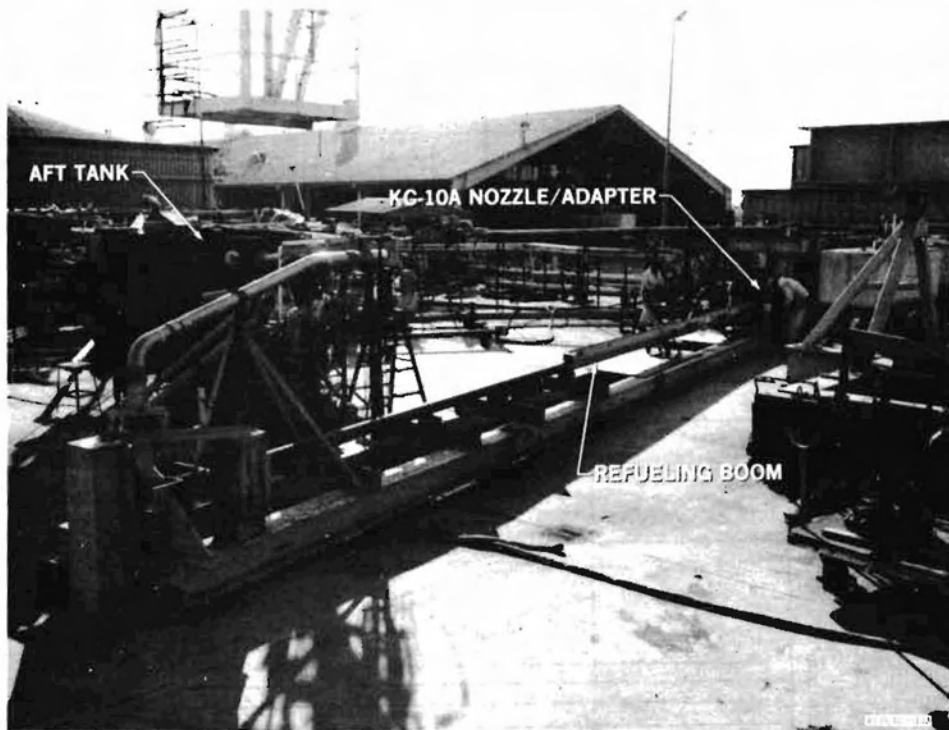
FIGURE 61. KC-10 AERIAL REFUELING SYSTEM SIMULATOR
