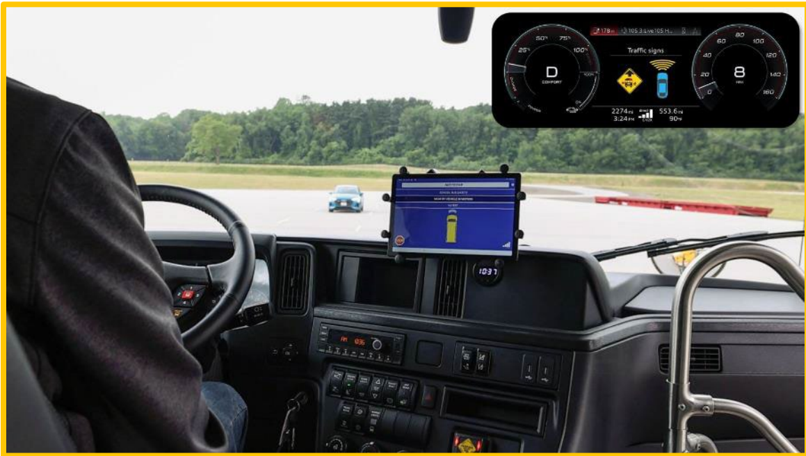
Figure 14: School bus and vehicle displaying safety information through C-V2X technologies
