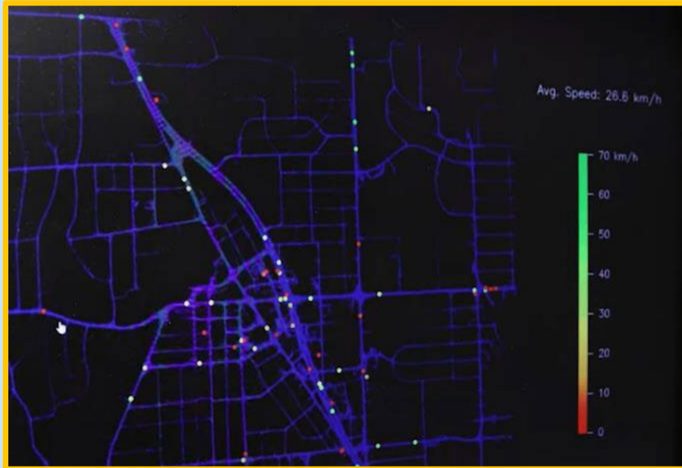
Figure 11: Example of vehicle trajectory data that displays CV speeds from the University of Michigan
