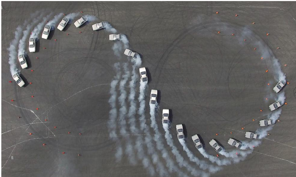
Autonomous vehicle drifting experiment at 50km/h, showing transitions through +/- 40 degrees sideslip in a second. (Image credit: Jonathan Goh. Source: https://news.stanford.edu/stories/2019/12/autonomous-delorean-drives-sideways-move-forward )
