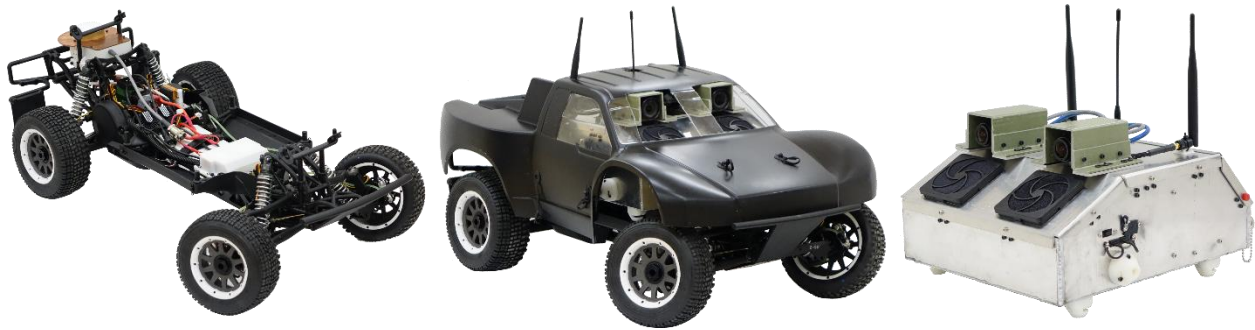
Figure 3.2 The AutoRally platform for testing aggressive high-speed self-driving, developed at Georgia Tech, led by Brian Goldfain, Paul Drews, and James Rehg (Williams et al., 2017)
