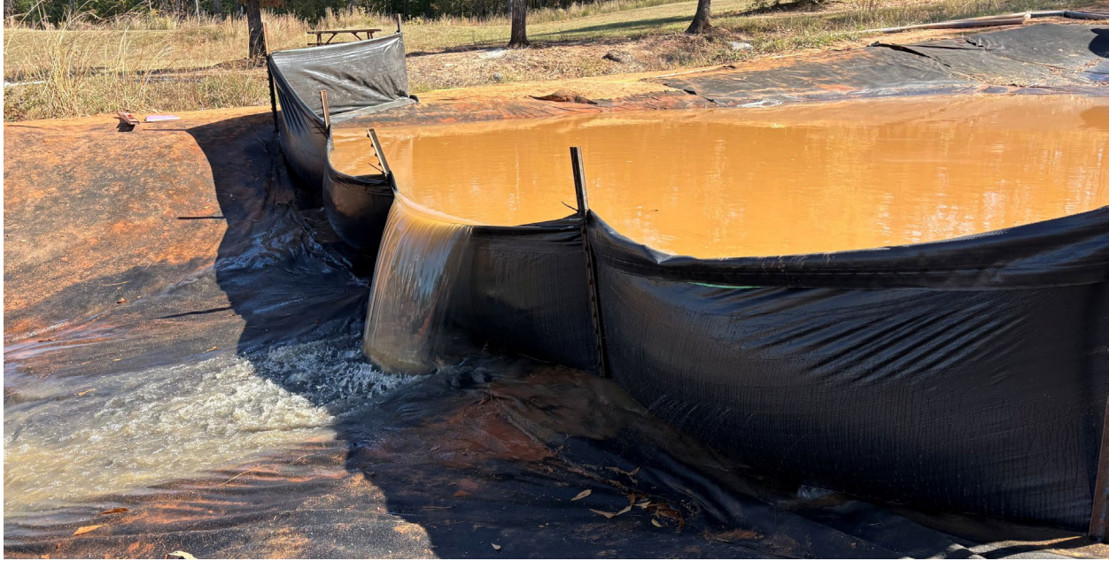
Figure 4.21: Installation 1 After Test C
