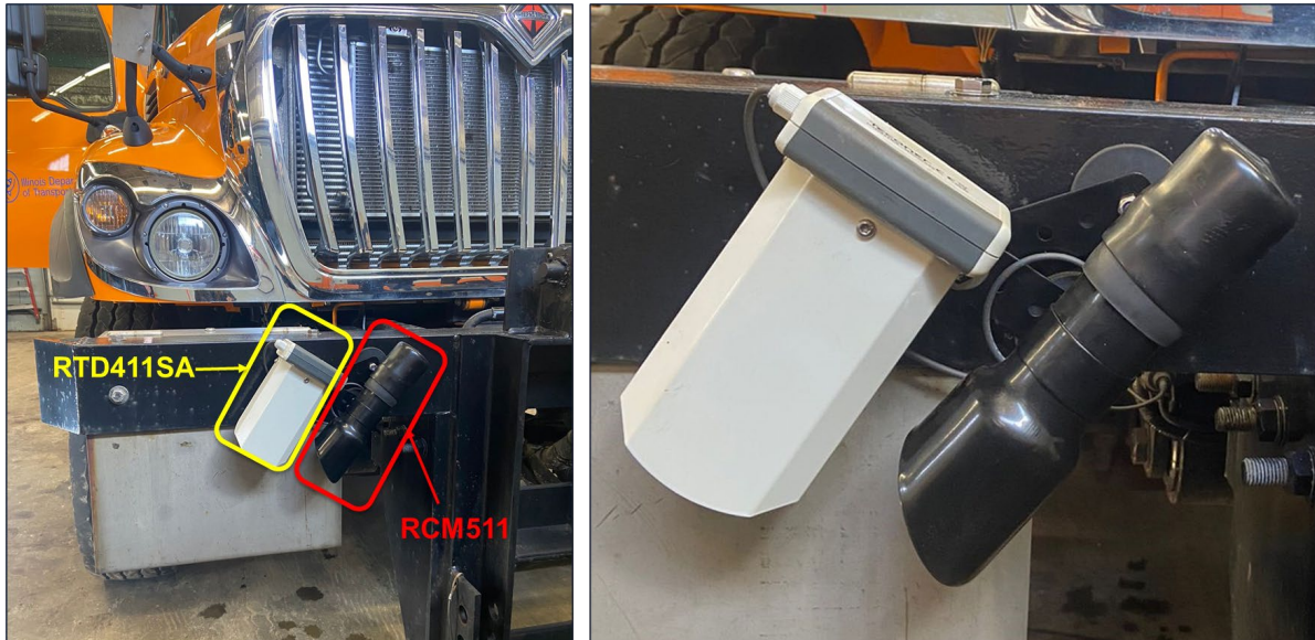
Figure 17. Photo. Mounting position of Teconer sensors on a snowplow.
