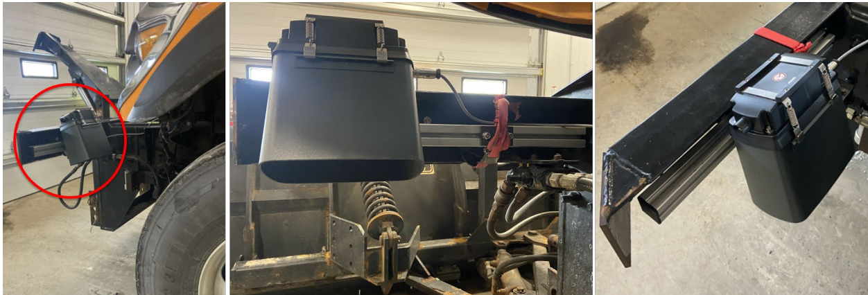
Figure 21. Photo. Mounting position of Lufft MARWIS unit on a snowplow.
