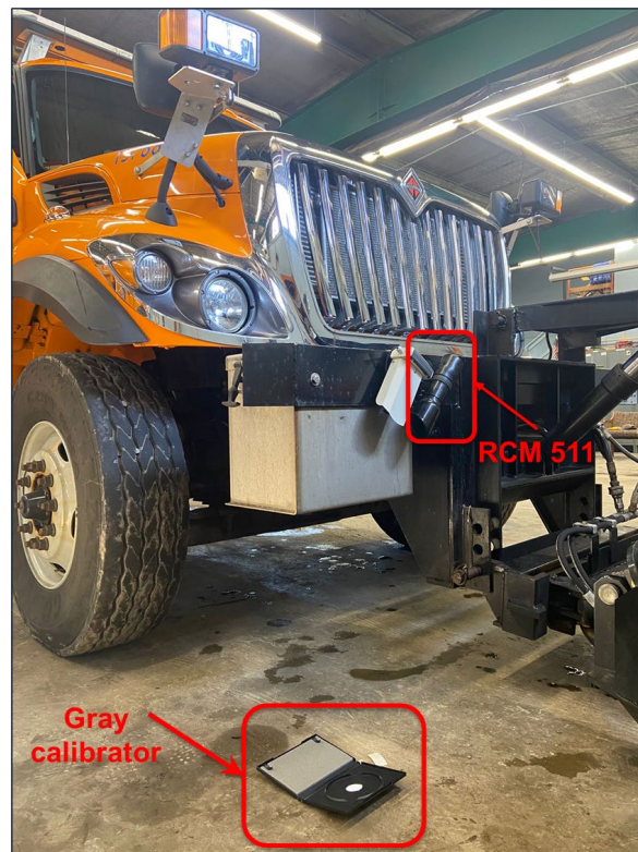
Figure 20. Photo. Calibration of Teconer system using gray calibrator.
