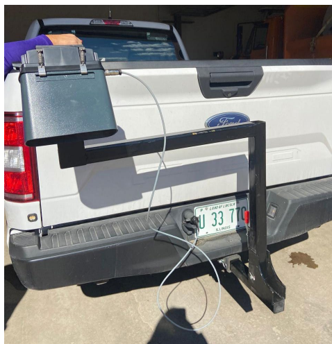
Figure 22. Photo. Mounting position of Lufft MARWIS unit on a supervisor vehicle.
