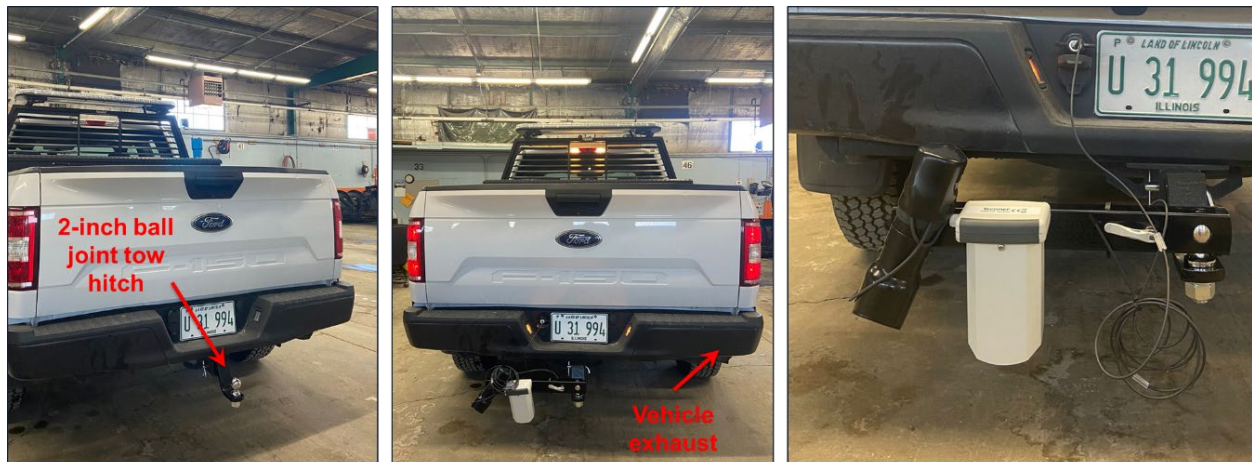
Figure 18. Photo. Mounting position of Teconer sensors on a supervisor vehicle.
