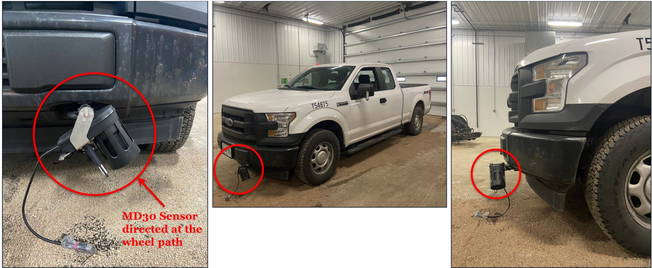
Figure 14. Photo. Mounting position of a Vaisala MD30 sensor on a supervisor vehicle.
