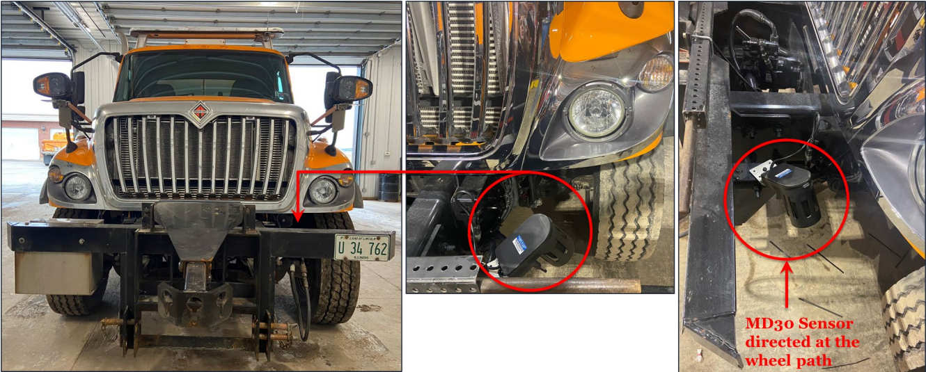
Figure 13. Photo. Mounting position of a Vaisala MD30 sensor on a snowplow.
