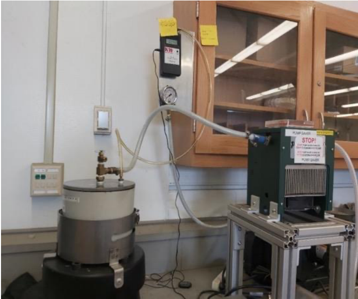
Figure 6. Vacuum Saturation of Conditioned Loose Asphalt Mixture and Shaker
