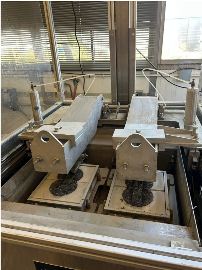
Figure 9. Hamburg Wheel Track Test Setup After Test
