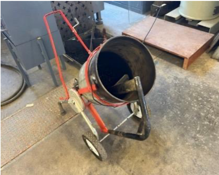
Figure 4. Mobile Mixer to Mix Aggregates with Binder
