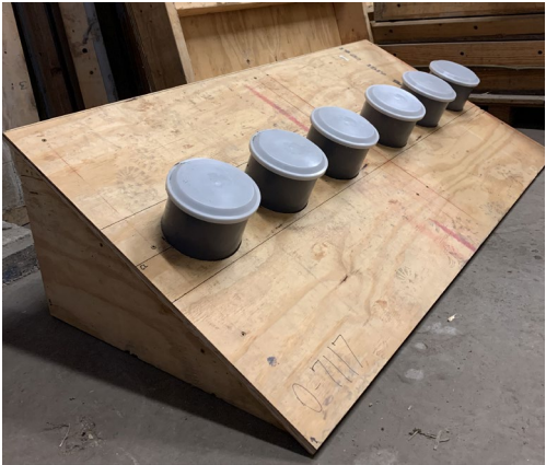
(a) Wood stand for 6×12-in. cylinders
