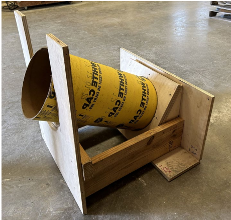
(b) Wood stand for 12×24-in. cylinder
