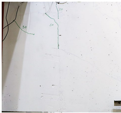
(a) Specimen photo at 50 kips
