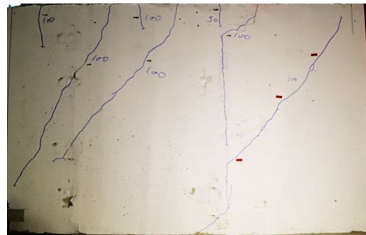
(b) Specimen photo at 100 kips
