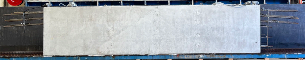
Figure 5-18 Interior section after the installation of dowel bars
