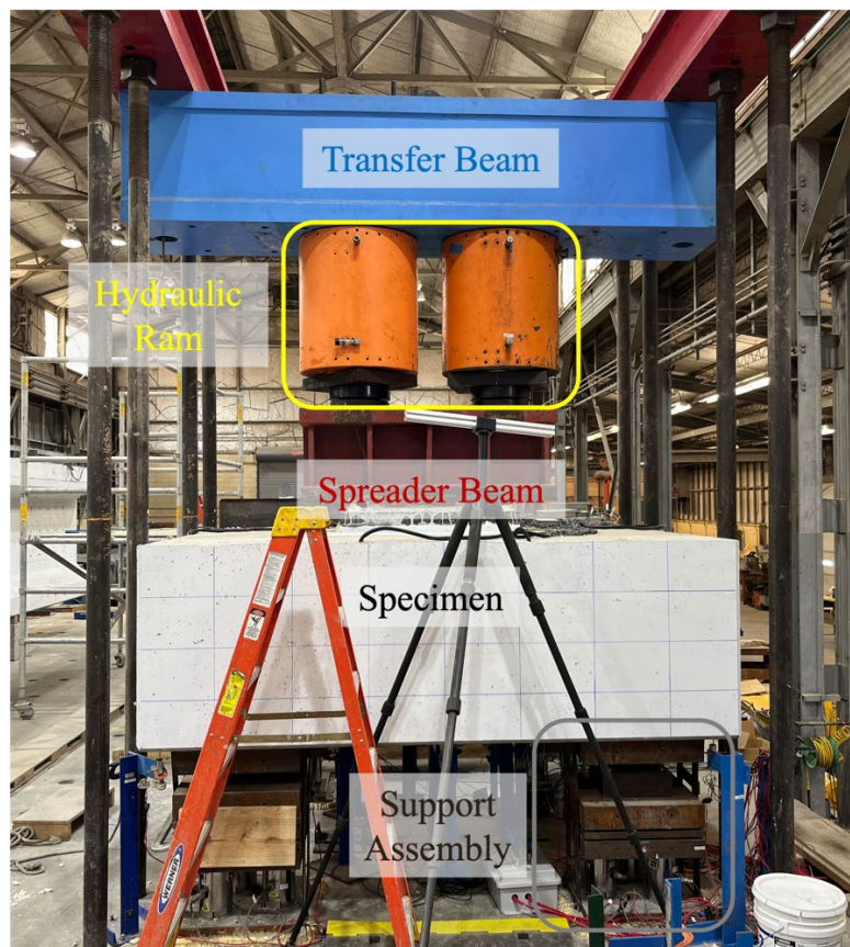
Figure 6-15 Test setup for drilled-shaft footing cap specimen
