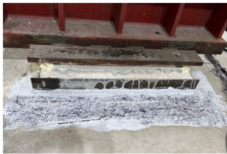
(a) Speckle pattern on the testing region
