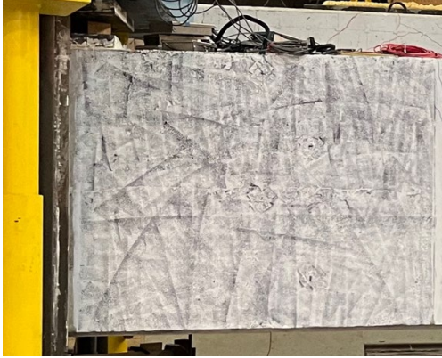
(a) Speckle pattern on the testing region
