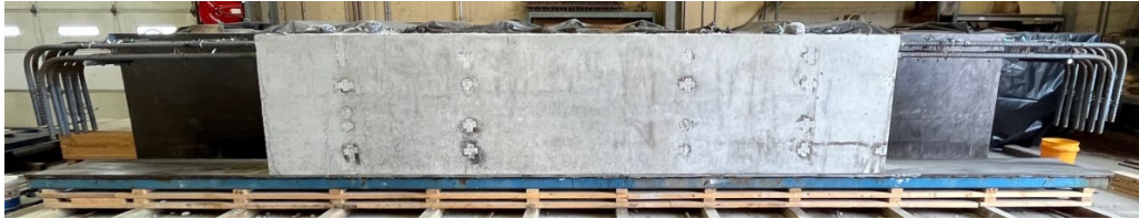
(b) Concrete cast in the interior section
