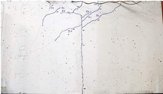
(a) Specimen photo at 50 kips
