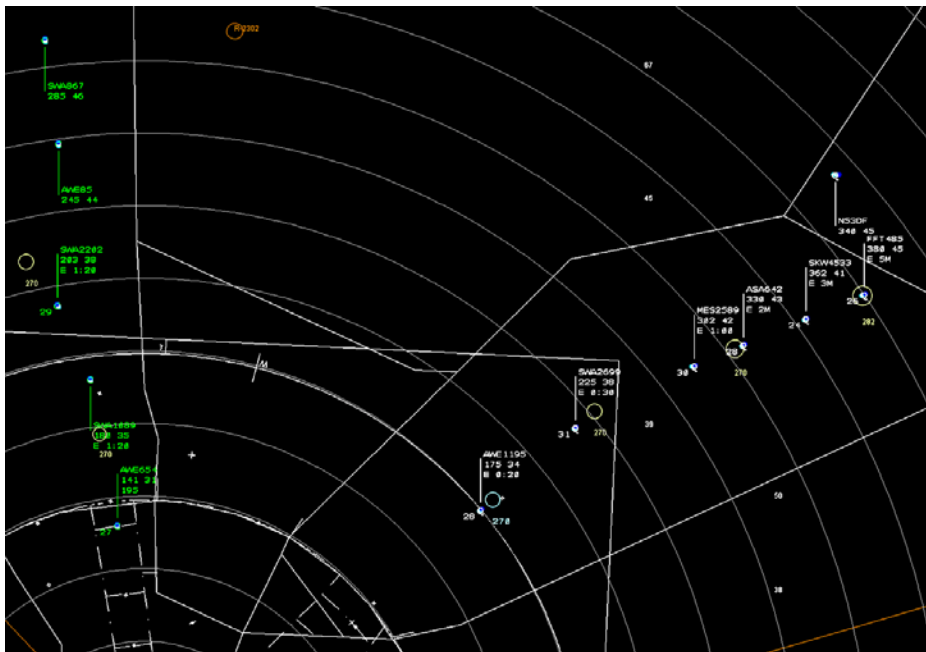
FIGURE 4.1.3-2. Pattern segmentation, as used on STARS to distinguish owned aircraft (white) from others (green).
