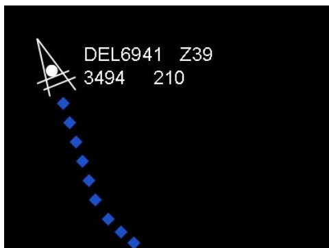
FIGURE 4.2.1-6. Redundant coding using color, shape, and position.
