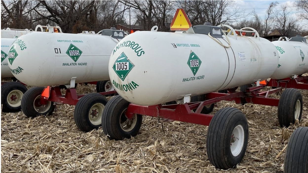
Figure 1. Nurse Tanks on Single Running Gear with Heads Extending Beyond Running Gear
