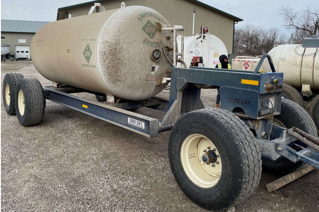
Figure 4. 3,000 gallon nurse tank
