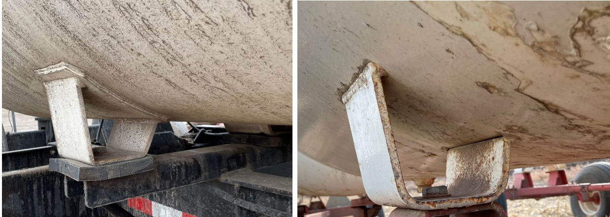
Figure 9. Edge-to-tank Foot attached via Pad (left) and Directly to Tank (right)
