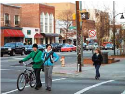
Crosswalks and pedestrian signals encourage pedestrians to cross at signalized intersections.
