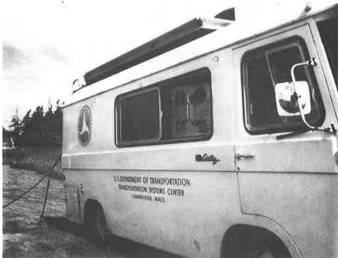
Figure 24. Cortez van equipped for lidar field test at Lubec. Transmitter and receiver optics can be seen through the side window
