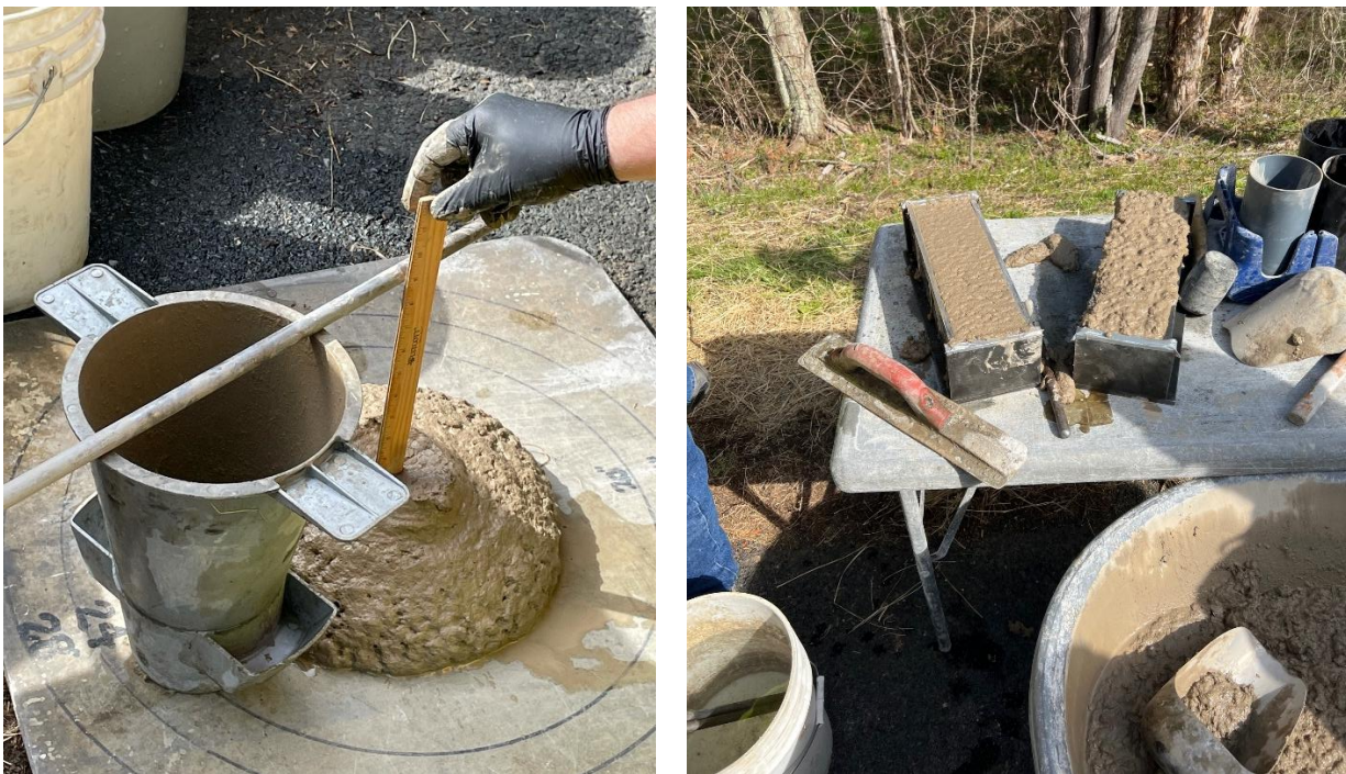
Figure 10. Photographs of Field Test: (a) Slump Test; (b) Sample Collection
