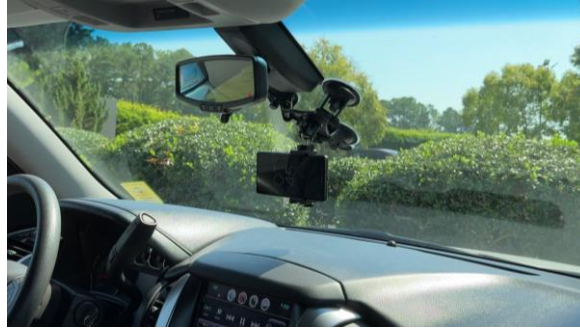
Figure 2. Photo. Example smartphone mounting setup
