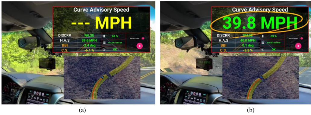
Figure 5. Photos. In-field advisory speed computation (a) before and (b) after curve exit
