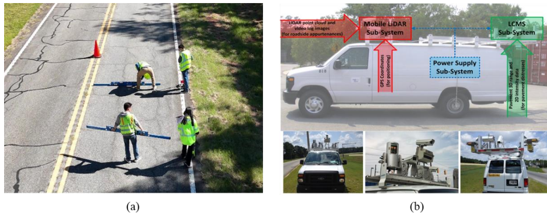
Figure 8. Photos. Reference cross-slope data collection, (a) manual, (b) 3D laser imaging
