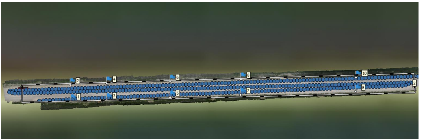
Figure 3. sUAS image points on 150th Street, Buchanan County, Iowa, with ground control points represented with flags
