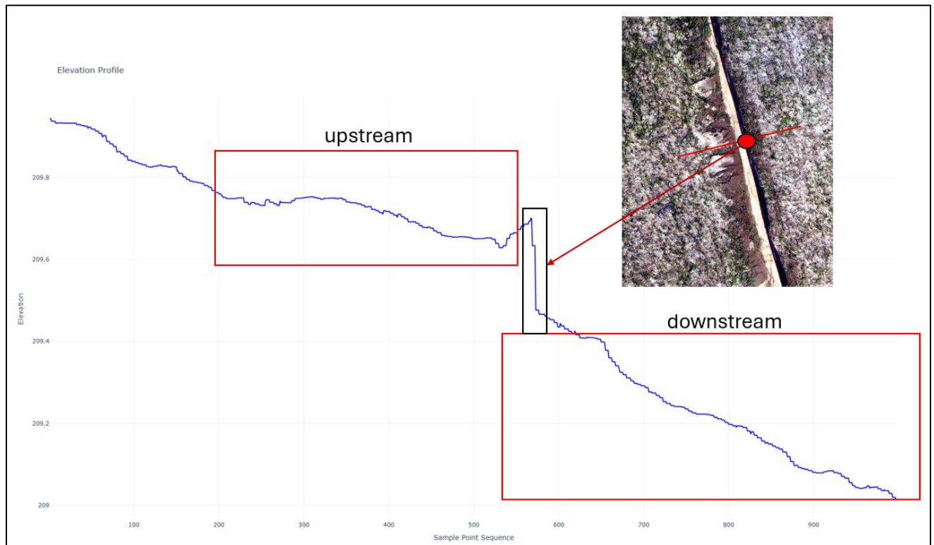
Figure 23. Plotted profile of a silt fence with accumulated sediment in the upstream section
