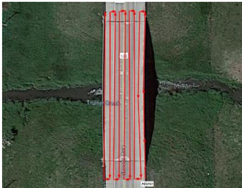
Figure 46. Manual mission flight at 15 ft (4.6 m) AGL
