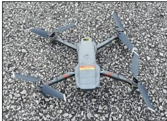
Figure 2. DJI Mavic 2 Enterprise Advance sUAS
