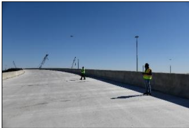
Figure 12. PIC controlling the sUAS while the VO keeps a close watch on the sUAS and the surrounding area
