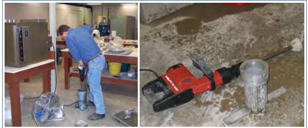
Figure 4-5. Molding RCC cylinder with vibrating hammer
