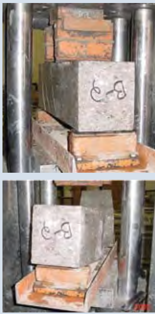
Test beam before (top) and after (bottom) testing
