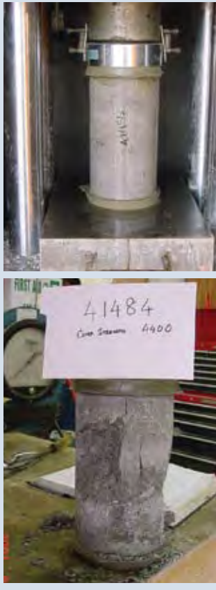
Compressive strength test cylinder before (top) and after (bottom) testing
