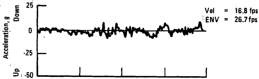
Figure 9-15. - Vertical decelerations resulting from first impact in 12° crash of R-5-0 Lodestar transport airplane.
