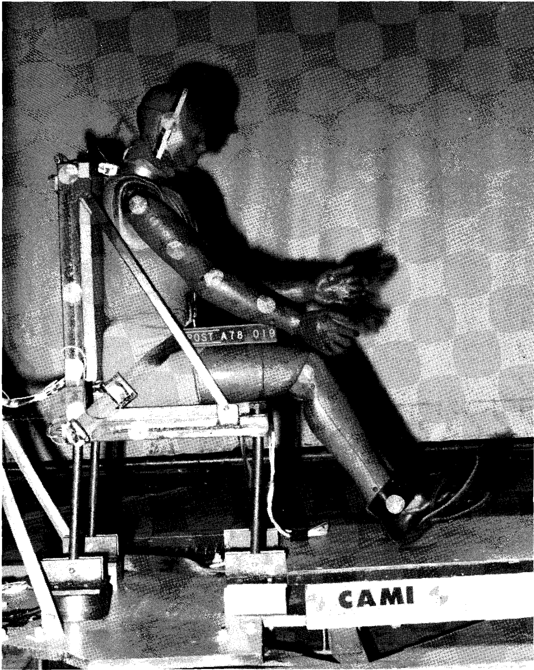
Figure 35. CAMI Series 2, low-deceleration, forward-facing test, posttest.
