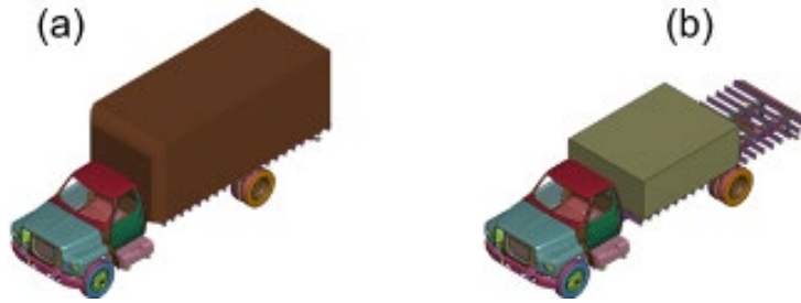
Figure 4.1: (a) Ford F800 SUT Finite Element Model, (b) Added Mass in Cargo Area
