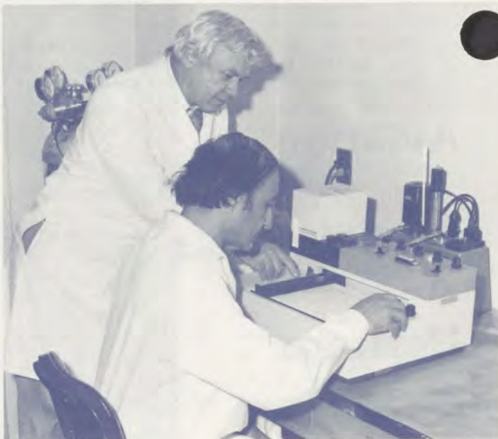
Dr. Jess McKenzie (standing) and chemist Russell Moses operate a Hem-O-Scan at CAMI to evaluate the interaction between oxygen and blood in disease studies.
