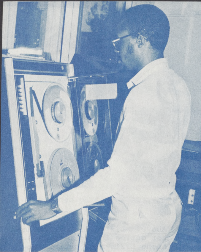
Left: Lonnie Hayes checking the tape which carries the information used in the printing of labels and envelopes on the addressing machine.
