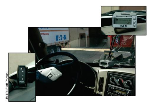
Figure 1. Driver-vehicle interface of the integrated safety system
