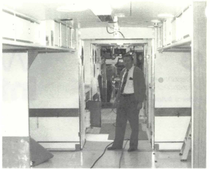
FAA Inspector Bruce Stuart checks bulkheads and storage closets in recovery room for security and proper placards.
