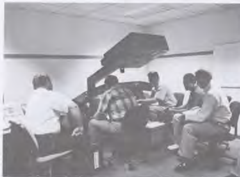
In the world of aviation simulation, this is known as a "device." A device provides no motion, nor any visuals out the cockpit windshield. In this instance, it is an instrument panel and that's all. The instructor develops the program on his computer, which then translates on the cockpit instruments in front of the trainees.
