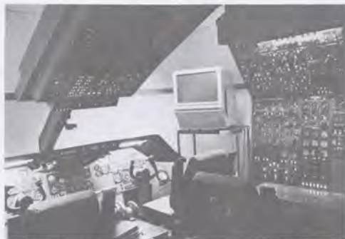
The full MD-80 cockpit "device" waits for a crew to be trained on flight operations systems, highly computerized in modern airplanes. It isn't necessary to have a full simulator to master the more complex cockpit systems before the simulator "flight."
