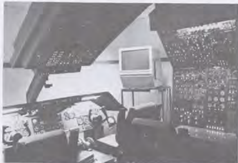
The full MD-80 cockpit "device" waits for a crew to be trained on flight operations systems, highly computerized in modern airplanes. It isn't necessary to have a full simulator to master the more complex cockpit systems before the simulator "flight."
