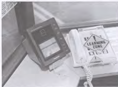
A cover over the telephone prevents mischievous fingers from dialing grandmother's house but does allow dialing the appropriate number to contact the air traffic control tower. Instructions located above the phone and the video camera explain how the system is activated.
