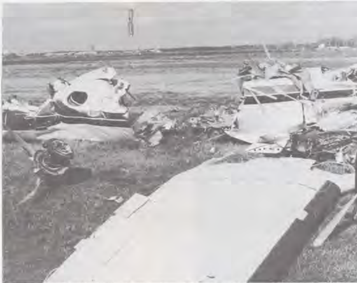
The bent propeller in the wreckage of N724N indicates it was spinning on impact. The wreckage was pulled by crane from Timbalier Bay, Louisiana. The plane was a Beechcraft King Air.
