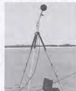
A microphone is installed for noise certification under Part 36.
