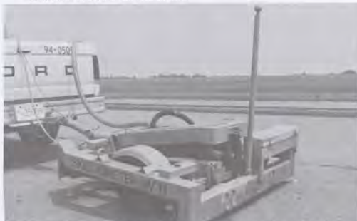
The BV-11 Skiddometer consists of a three-wheel trailer towed behind a vehicle. Equipped with an on-board water delivery system, the tester can be operated at speeds up to 100 mph.
