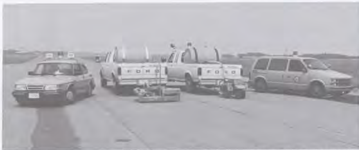
FAA-approved friction measuring equipment (left to right): Saab Friction Tester, BV-11 Skiddometer, Mu-Meter, and Low Friction Tester.
