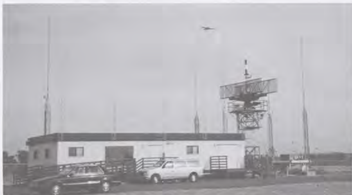
The test facility at Memphis shows the back-to-back Mode S or secondary radar antenna. The displays are in the trailer where the test exercises are run.
