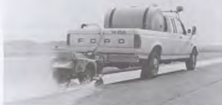
The ML Aviation Mu-Meter performs tests on simulated ice.
