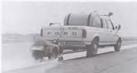
The Saab Friction Tester incorporates a fifth wheel mounted behind the rear axle of the vehicle. This wheel is driven by a chain transmission connected to the rear axle.
