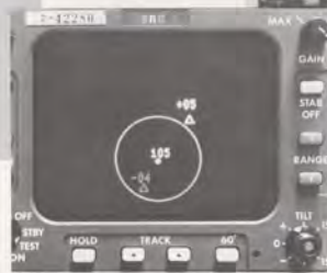
A TCAS II-equipped aircraft is shown at the center of a two-mile range ring at 10,500 feet. An "intruder" at seven o'clock is 400 feet below the TCAS II plane, while another aircraft is shown 500 feet higher.
