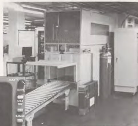
The thermal neutron analysis bomb detector has the ability to search for specific combinations of atomic elements that characterize explosives.
