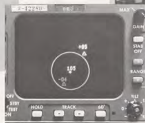
A TCAS II-equipped aircraft is shown at the center of a two-mile range ring at 10,500 feet. An "intruder" at seven o'clock is 400 feet below the TCAS II plane, while another aircraft is shown 500 feet higher.
