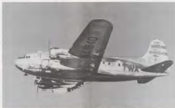
The Boeing 307B Stratoliner was the first airliner with a pressurized cabin and the first with four engines.
