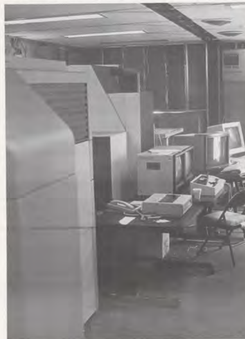
Moving day shows the many pieces of the machinery beginning to take shape (top and bottom photos). Before this machine was built, several prototypes were tested at San Francisco and Los Angeles airports. More than 40,000 bags were screened.
